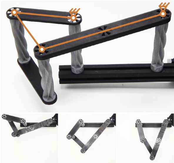
Fig. 7. A neutrally stable four-bar linkage (orange schematic) is constructed with rigid links (black) and helicoidal shell joints (grey). The joints are preloaded such that they act in their constant moment range. At the bottom, top-views of a number of equilibrium positions are shown. See Supplementary Video 3.
