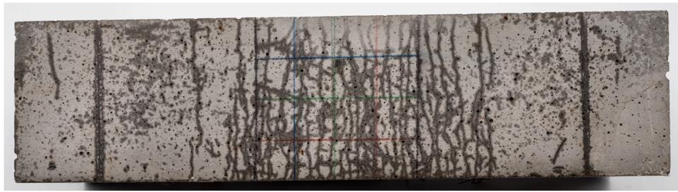
Fig. 10. Multiple micro-cracking formations in flexural harding stage (micro-cracks revealed by alcohol spayed on the surface).
