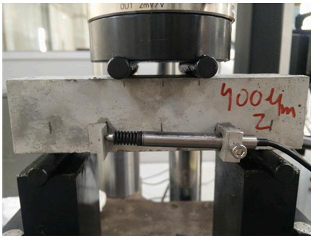
**Fig. 1.** Four-point bending test.
