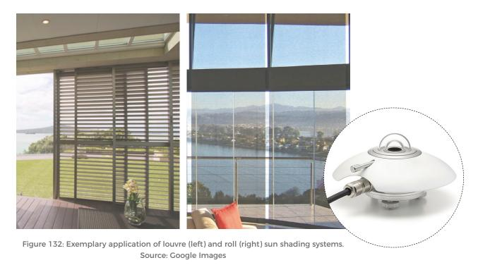
Figure 133: Pynanometer. A device that measures solar irradiation. Source: Google images
