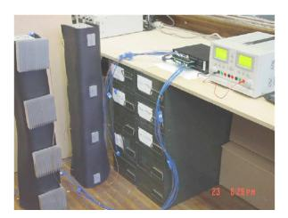
Figure 97: (left) Testing room model for performance test. Source: Xu et al. Figure 98: (right) Experimental setup for performance test. Source: Xu et al.
