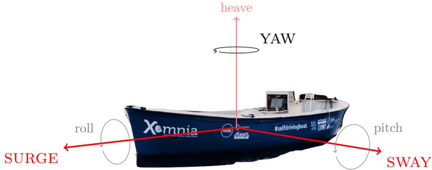
Figure 2.3: 6 DOF motions. The capitalized motions are considered for the 3DOF coordinate system. The red motions are translational motions and the black motions are rotational
