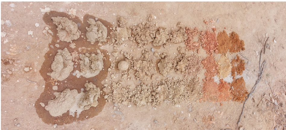
Figure 3.6: Soil samples at the drilling site. The samples are sorted according to depth with the top right sample being the first drilling meter to the bottom left sample at 33 m going column by column. The iron oxidation and visible changes in particle size distribution guided the decision of which samples to analyze.
