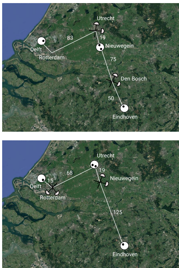
Figure 6.7: Two possible choices for processing node (white circles, black circles within represent qubits) and heralding station placement in the SURF network's shortest connection between the Dutch cities of Delft and Eindhoven. In the path on the left, the Rotterdam node is unused, thereby directly connecting the Delft - Rotterdam and Rotterdam - Utrecht links. Similarly, the Den Bosch node is unused in the path on the right.
