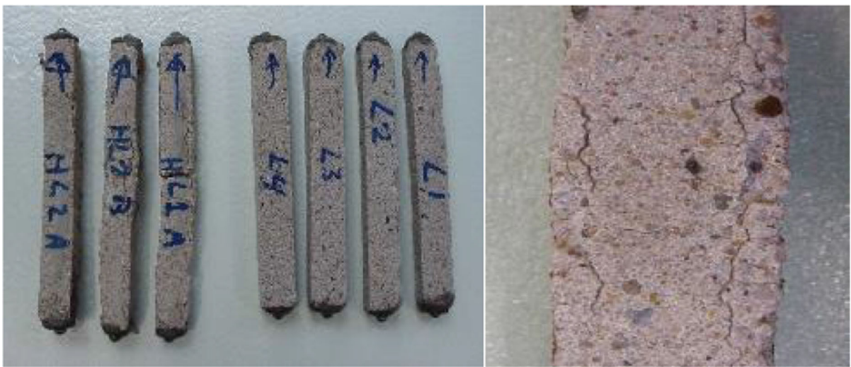
Fig. 20 Mortar prisms after 15 weeks in sulfate solution. Natural Hydraulic Lime based (NHL) specimens with clear expansion and deformation and Hydrated lime based (CL)
