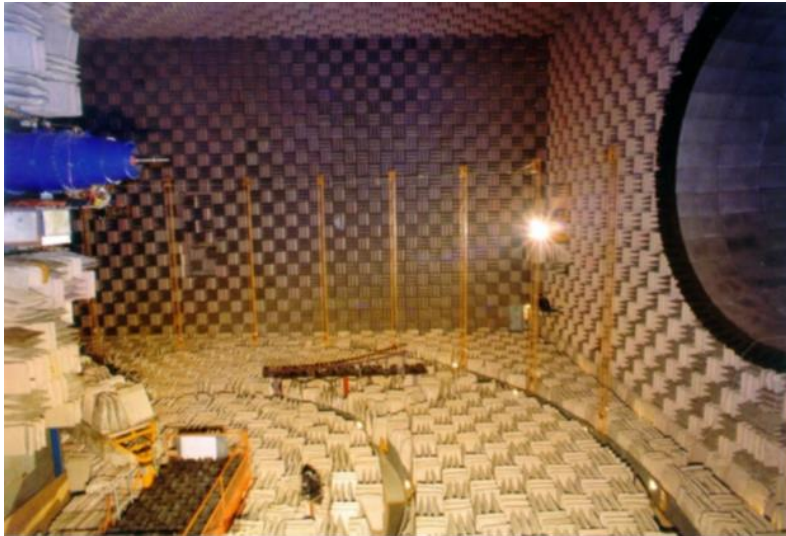
Figure 3: The free-jet, jet nozzle and far-field microphones in the QinetiQ Noise Test Facility
