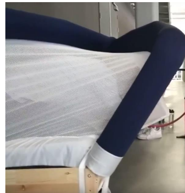
Figure 30 Behavior of the CloudCuddle Junior shows there is fixation on the bottom of the tube and it leans over.
