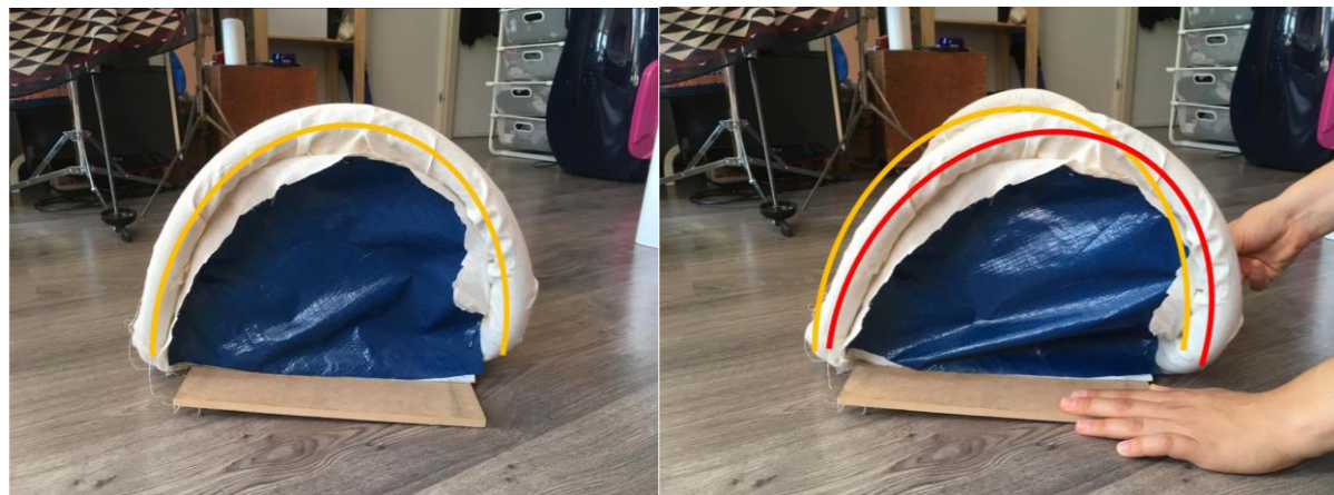
Figure 40 A simple test with a scaled prototype shows that the inflatable tubes deform, although the side material is not mesh but a fabric with minimum elasticity.
