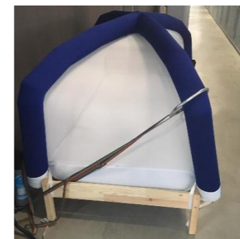
Figure 33 A quick solution to test the hypothesis that a fixating the tube would prevent the inflatable tube from bending over.
