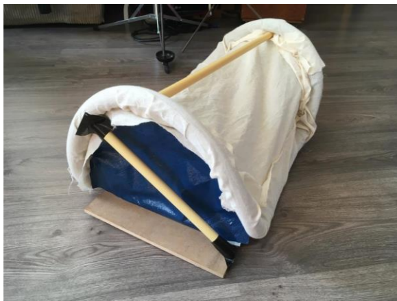
Figure 45 The mock-up scale with it's diagonal poles and top pole that made the inflatable tubes more stiff.
