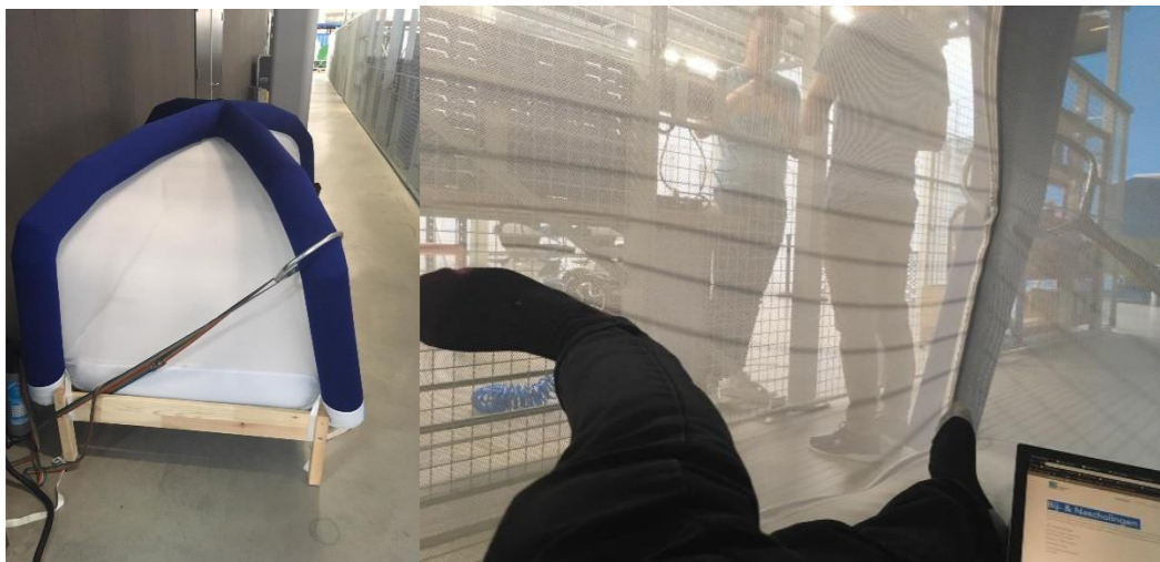
Figure 48 Fixating the inflatable tube made the mesh more stiff.
