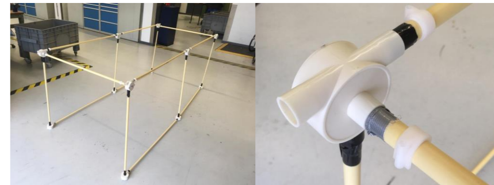
Figure 54 A low, midhigh and high frame of PVC was made to test with participants.
