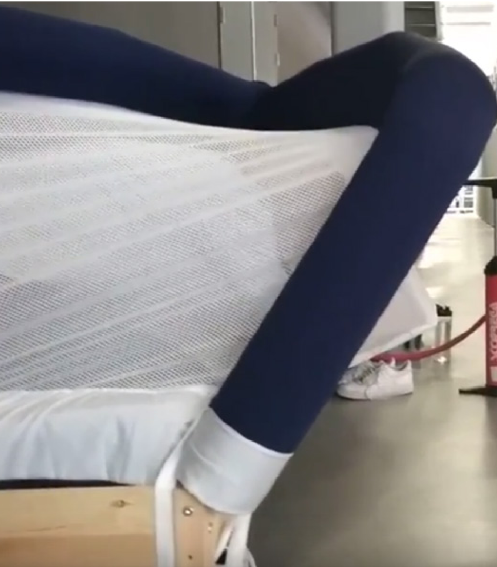
22 figure 11. When pushed against, CloudCuddle Junior tips over due to a lack of fixtures.
