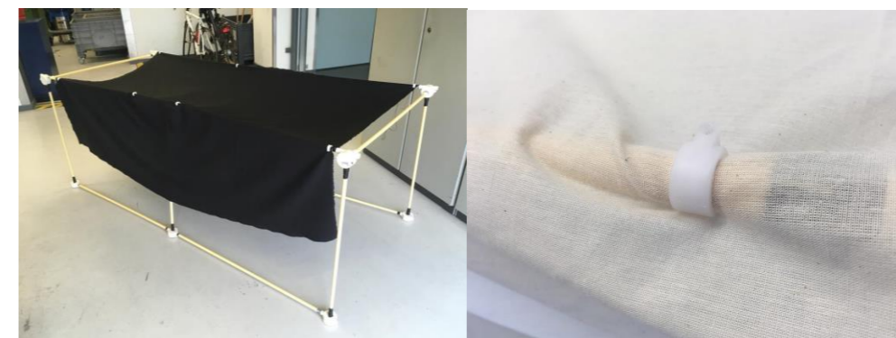
Figure 55 Dark and Light Fabric and Mesh could be fixated to the sides and on top.
