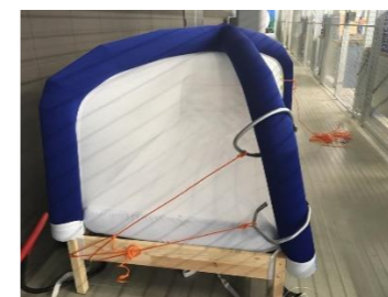
Figure 34 Fixating the inflatable tube with 2 ropes made the structure more stiff. It was assumed that this was enough.
