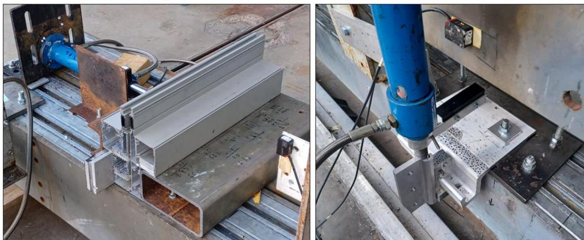
Figure 3.11 Connection test. Left: Transom-transom in-plane. Right: Top aluminium bracket and hook
