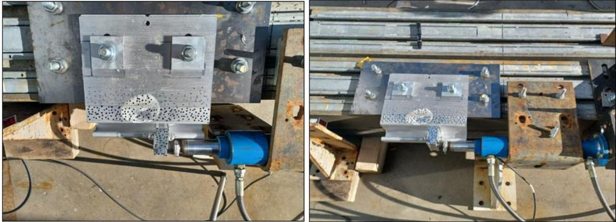
Aluminium bracket horizontal. Load on bracket
