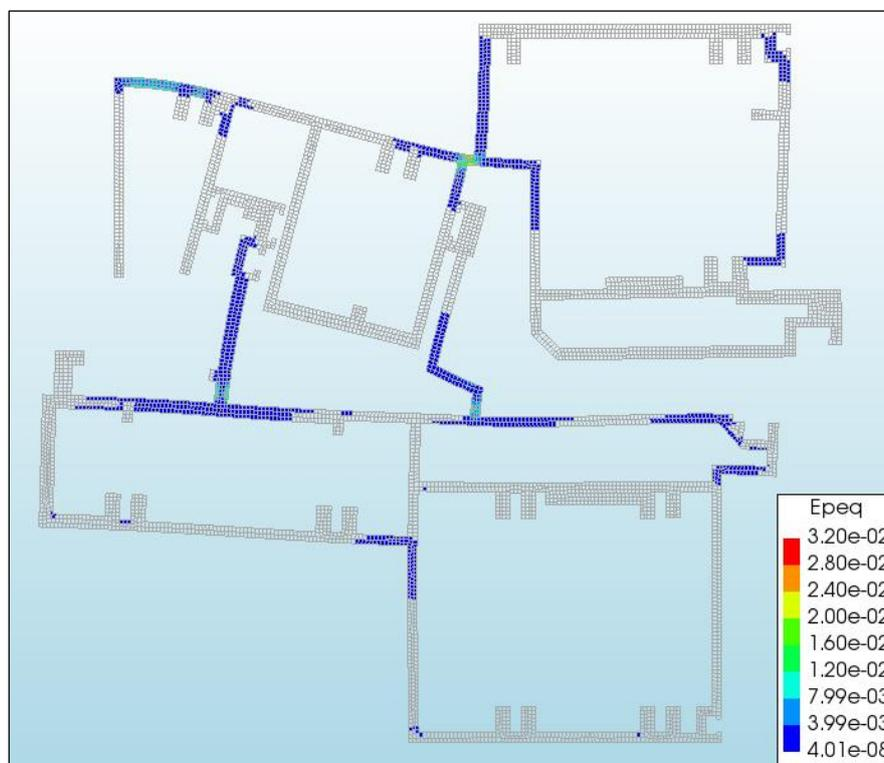
Figure 4.23 Transom-starter sill out-of-plane outwards. Final deformed shape and plastic strains.
