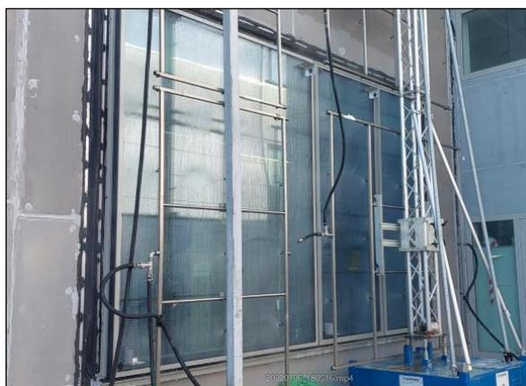
Figure 3.12 Water penetration resistance – static pressure test
