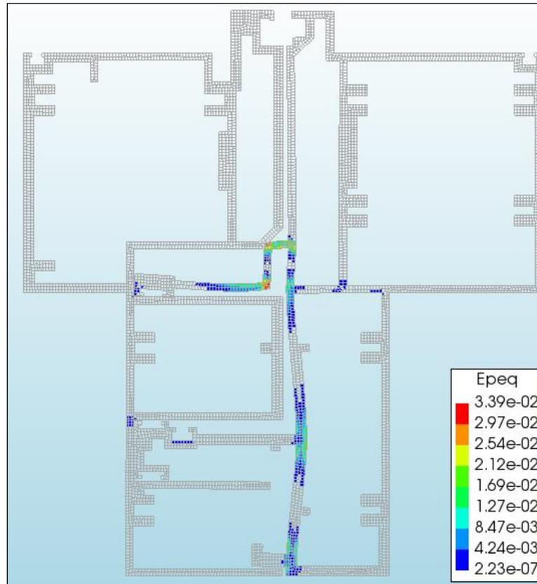
Figure 4.20 Transom-Starter sill in-plane. Final deformed shape and plastic strains.
