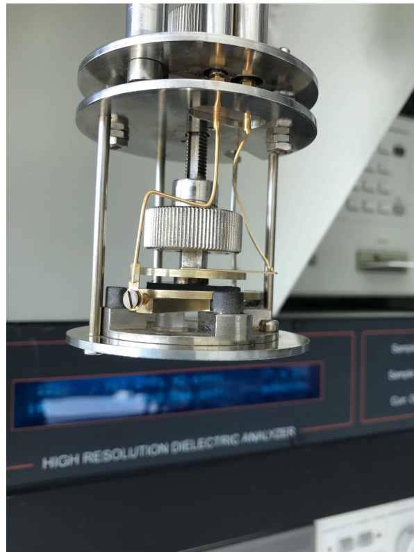
Figure A.7: Example of a cut and sputtered sample loaded into the BDS sample cell. It can be noted that on top of the sample an additional small electrode has been placed.
