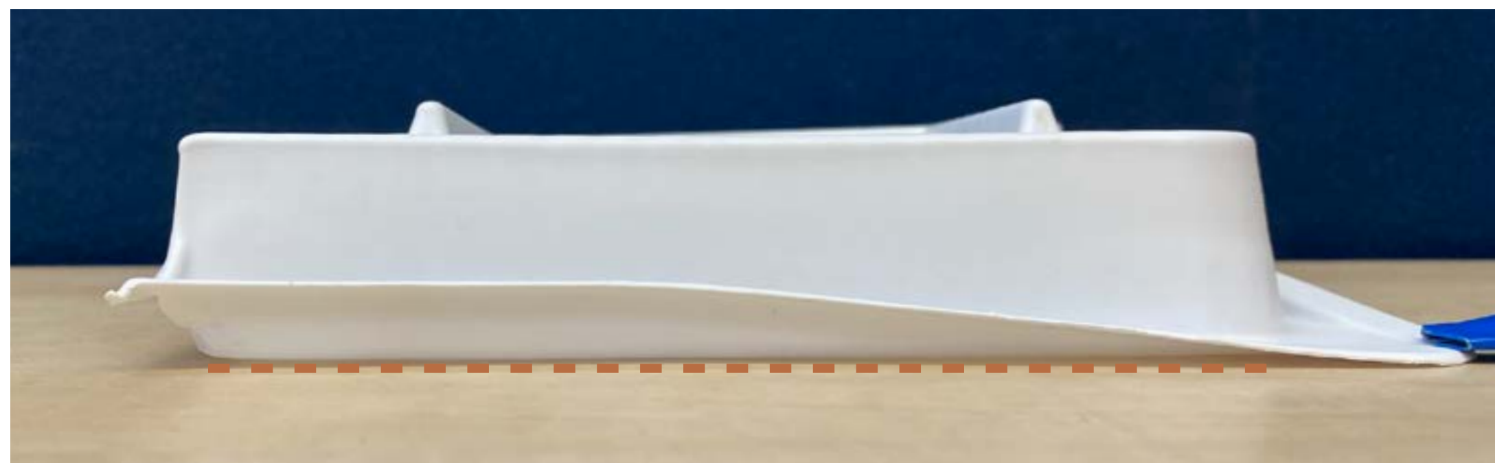
Figure 105. Result from thermoforming. The outer edge has reached all the way into the bottom of the mold gutter, resulting in a straight bottom (indicated by the brown dashed line).
