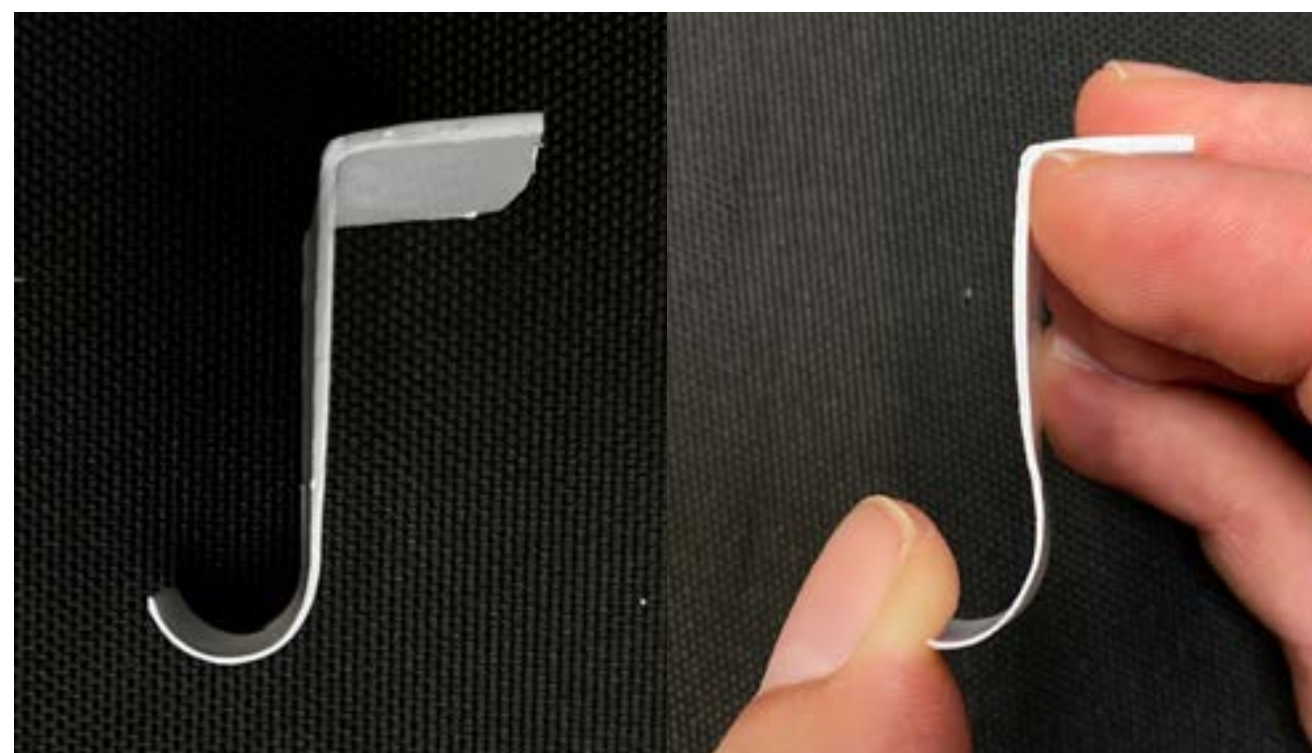
Figure 108. The PS sheet gets thinner toward the bottom of the mold gutter. It therefore bends quite easily.
