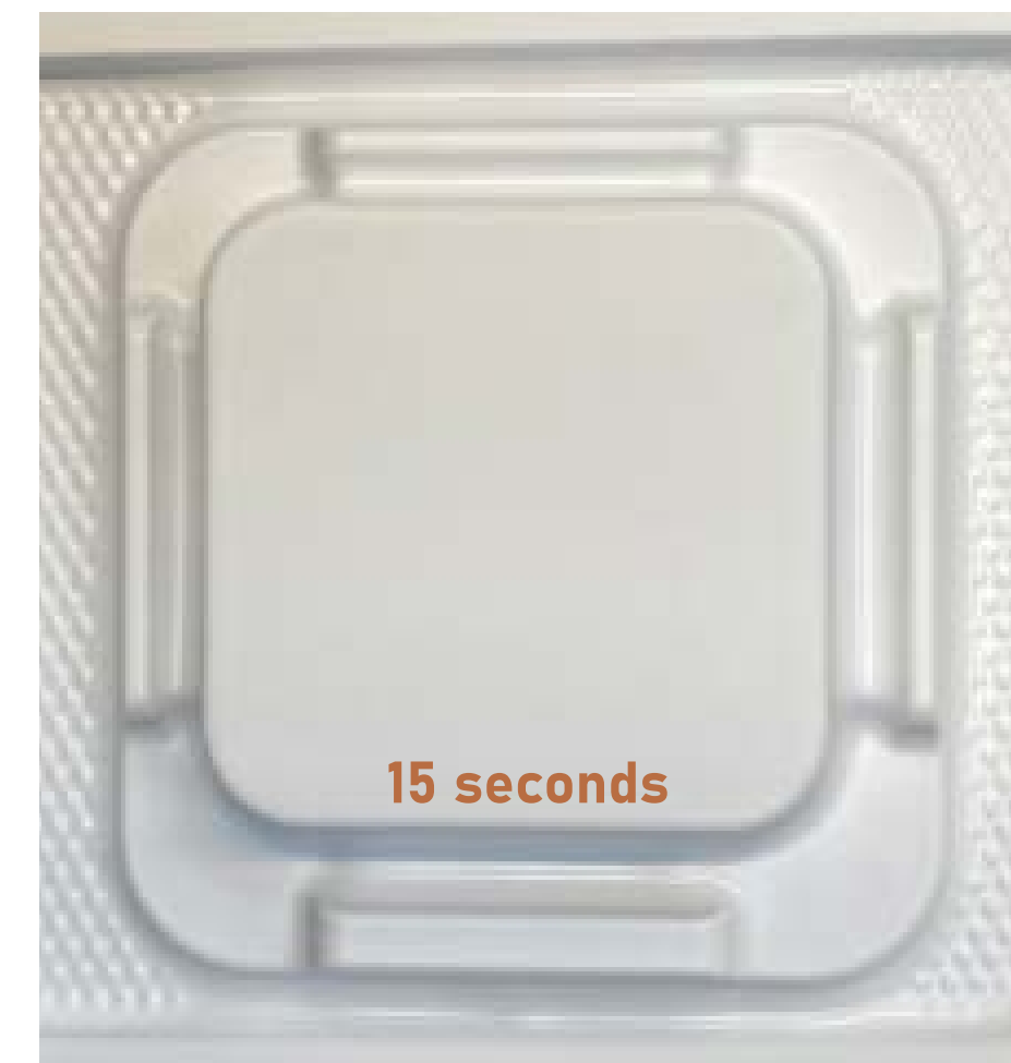
Figure 101 (left). Thermoforming was successful for the 10, 12 and 14 mm wide gutters. The material did reach the bottom of the 7 mm wide gutter, but also formed rockets at both ends of the edge.
