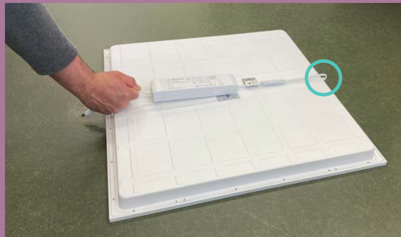
Figure 72. Demonstration of the driver pull test. The cable to panel connection circled in blue may not be disturbed.
