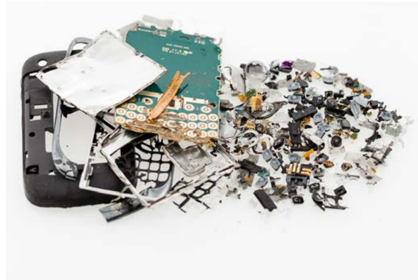
Figure 17. Mobile phone disassembled through pulsed power (ImpulsTec, n.d.-a).
