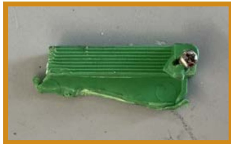
Figure 40. Steel screw still stuck in CoreLine connector housing.
