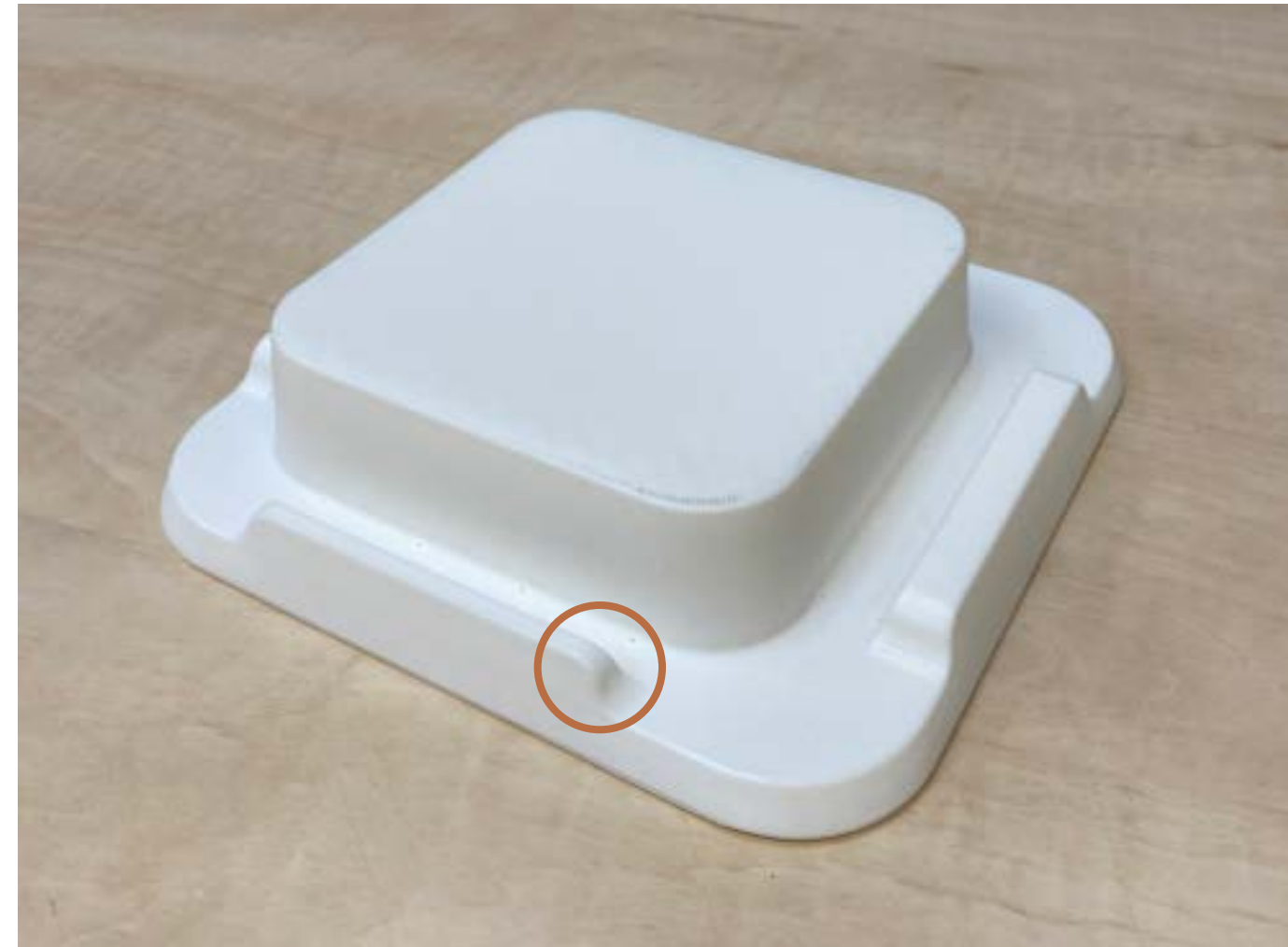
Figure 100. 3D printed mold for testing edges with different gutter widths. The ends of the edges have been given a larger rounding (indicated by brown circle).
