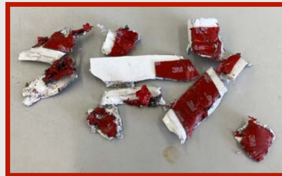
Figure 41. Sticker still stuck to CoreLine driver housing.
