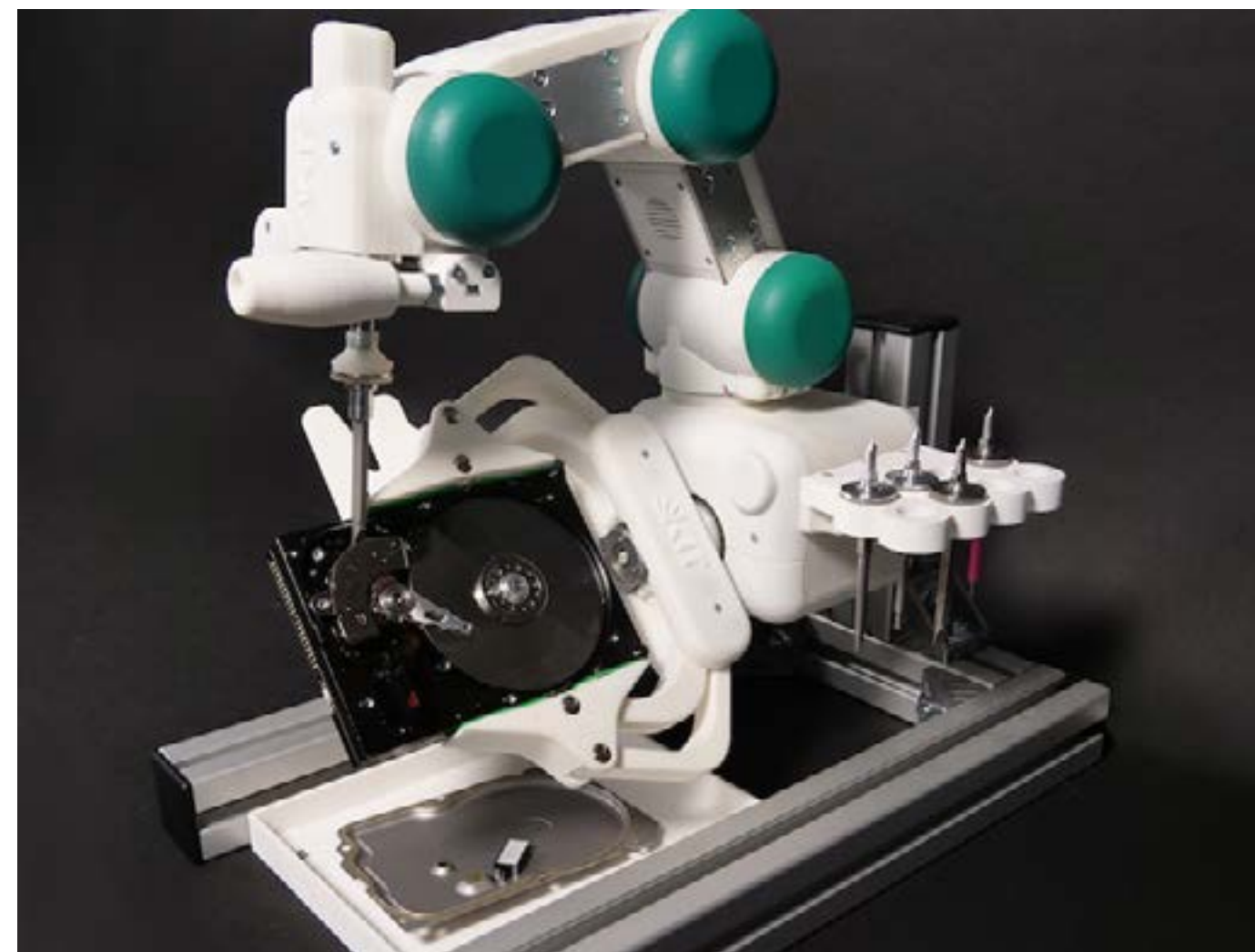
Figure 18. IMAGINE robot dismantling a hard disk drive. © Gripper_Karlsruhe Institute of Technology IAR-H2T.
