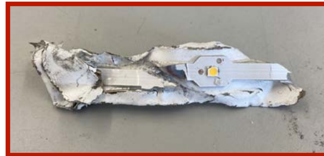
Figure 48. Mixed fragment of L2 and steel backplate as a result of glue.
