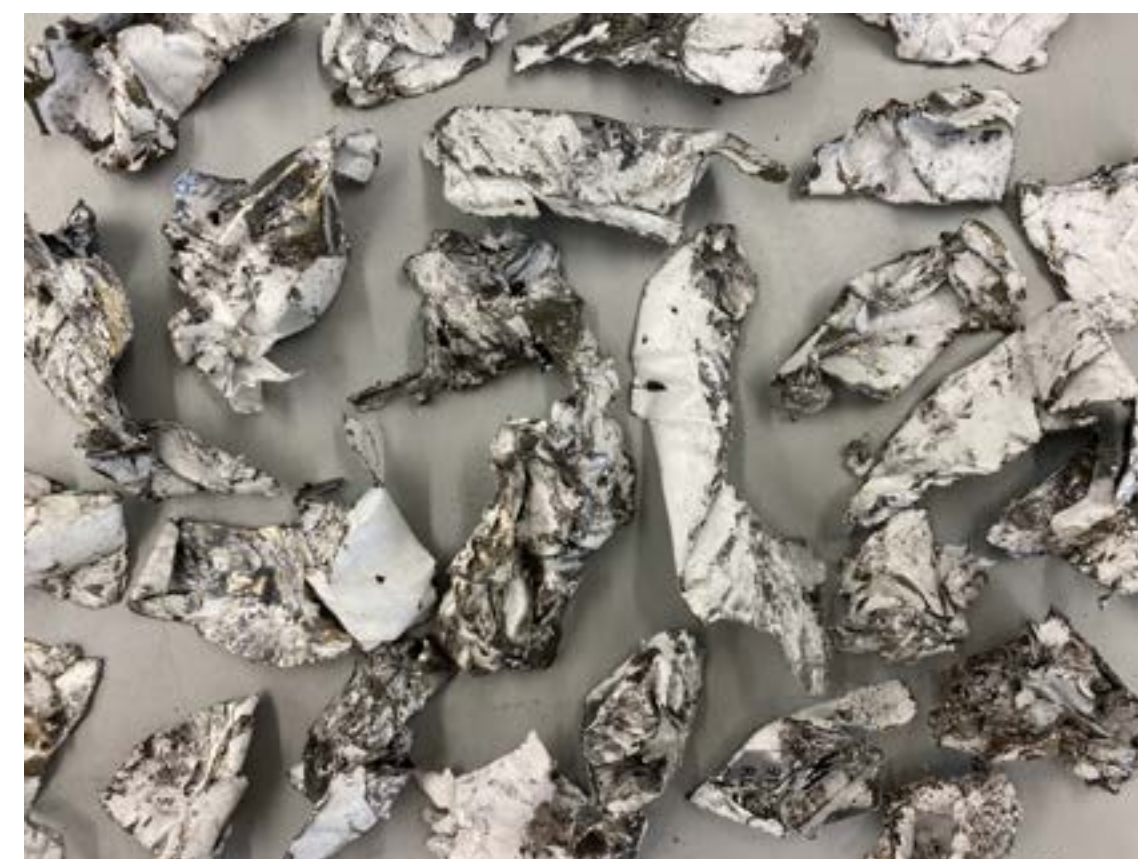
Figure 81. Steel backplate is prone to folding during shredding.
