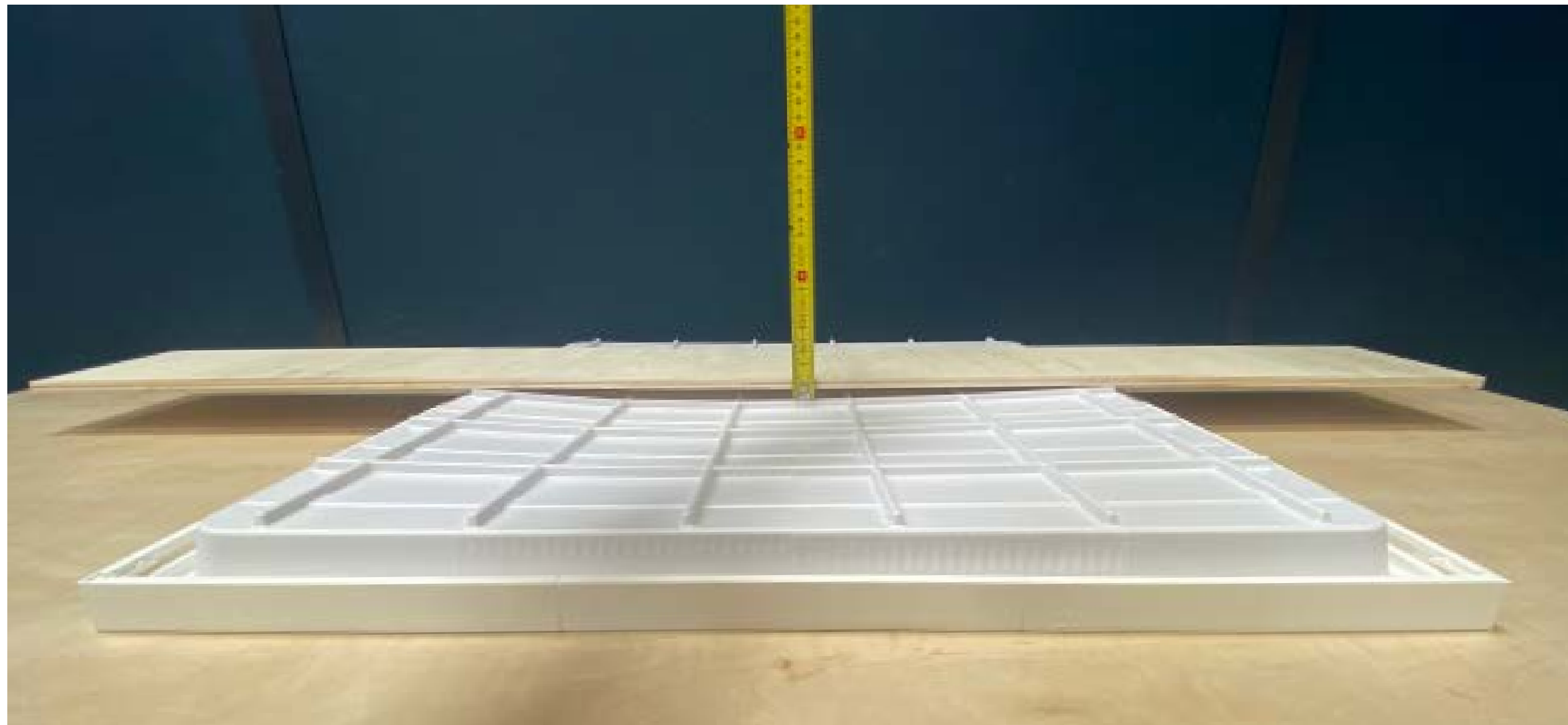
Figure 139. Maximum deflection of the backplate is 10 mm.
