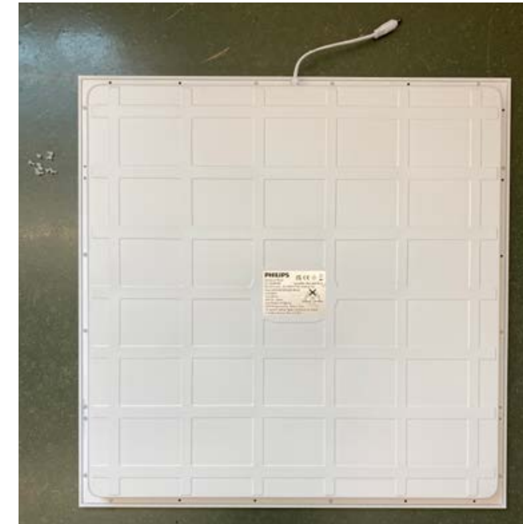
Figure 62. Half of the plastic screws fell out of the backplate when turned upside down.
