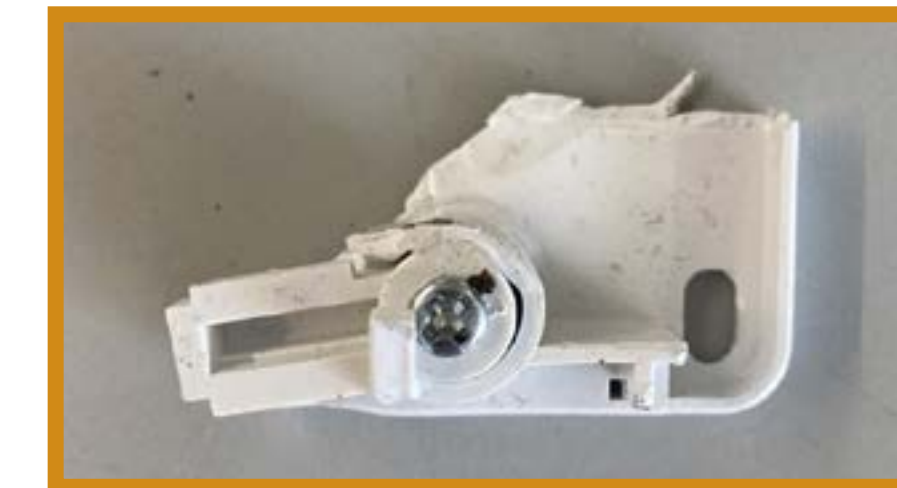
Figure 38. Steel screw still stuck in CoreLine driver housing.
