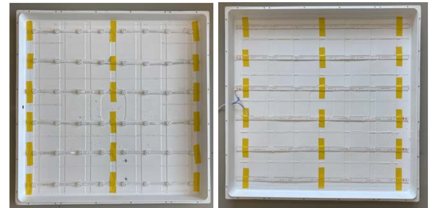
Figure 82. Prototypes to test if L2s will get wrapped up in steel backplate when they are not glued. Left: aluminum L2s. Right: epoxy L2s.
