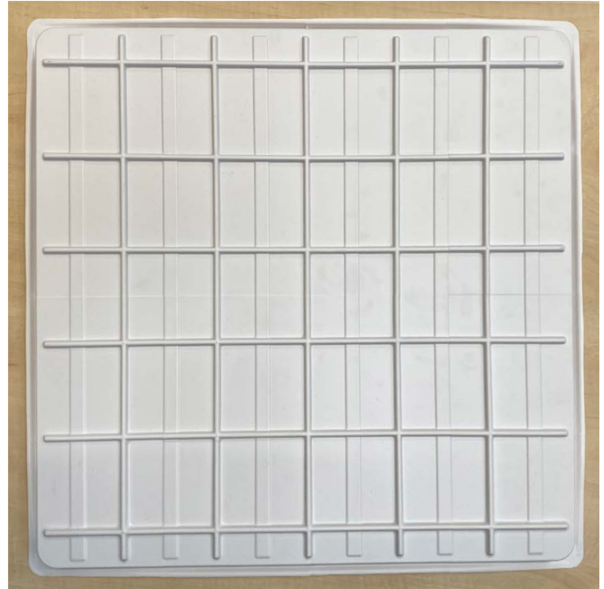
Figure 107. Thermoformed backplate in 1:1 scale.
