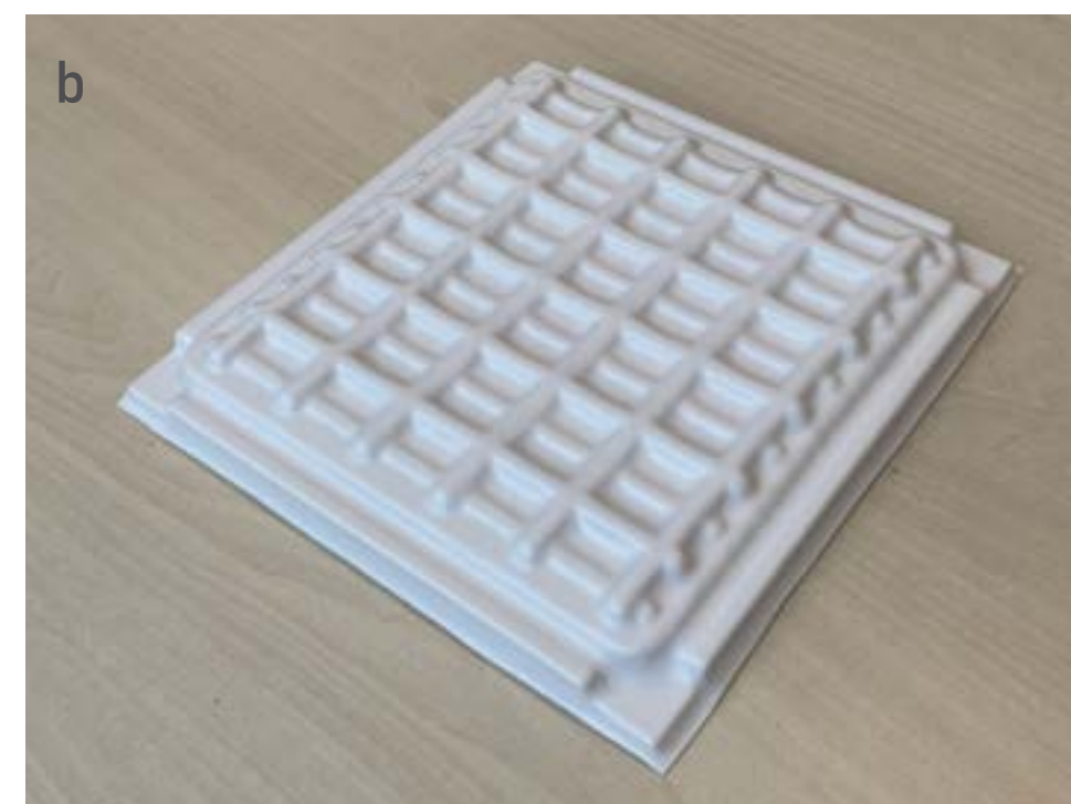
Figure 94. (a) 3D printed mold of 1:3 backplate. (b) result from thermoforming.
