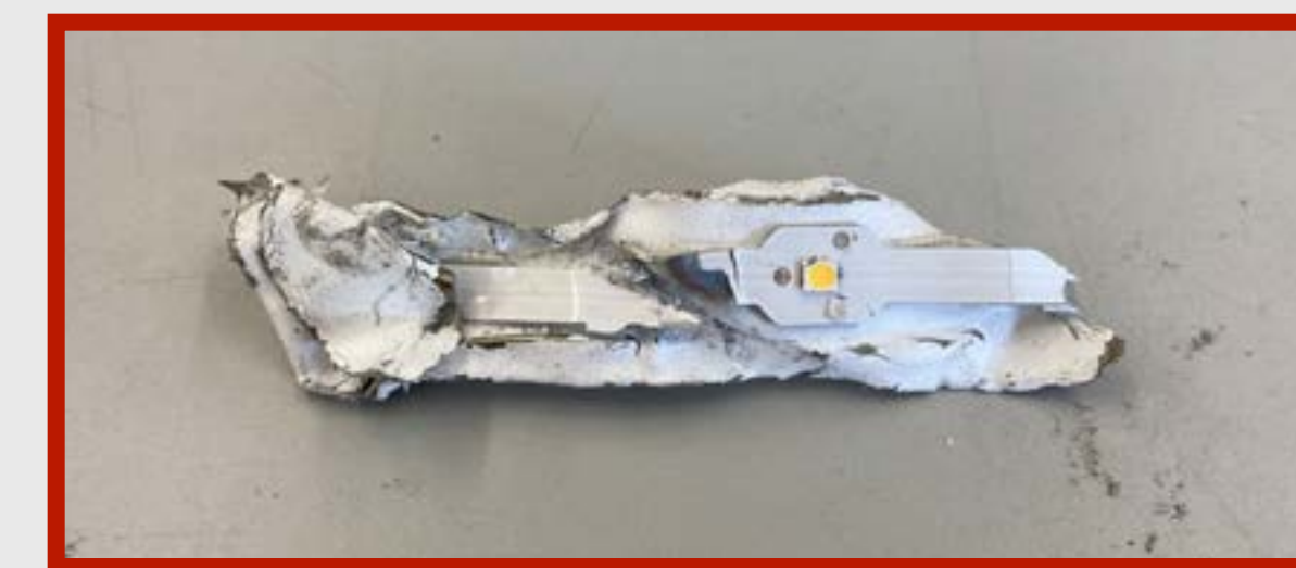
Figure 34. L2 still stuck to steel backplate in CoreLine.
