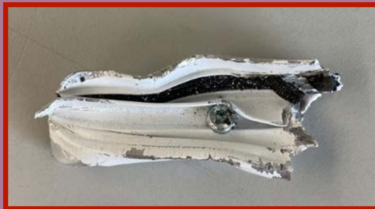
Figure 61. Mixed fragment of aluminum frame and steel screw.
