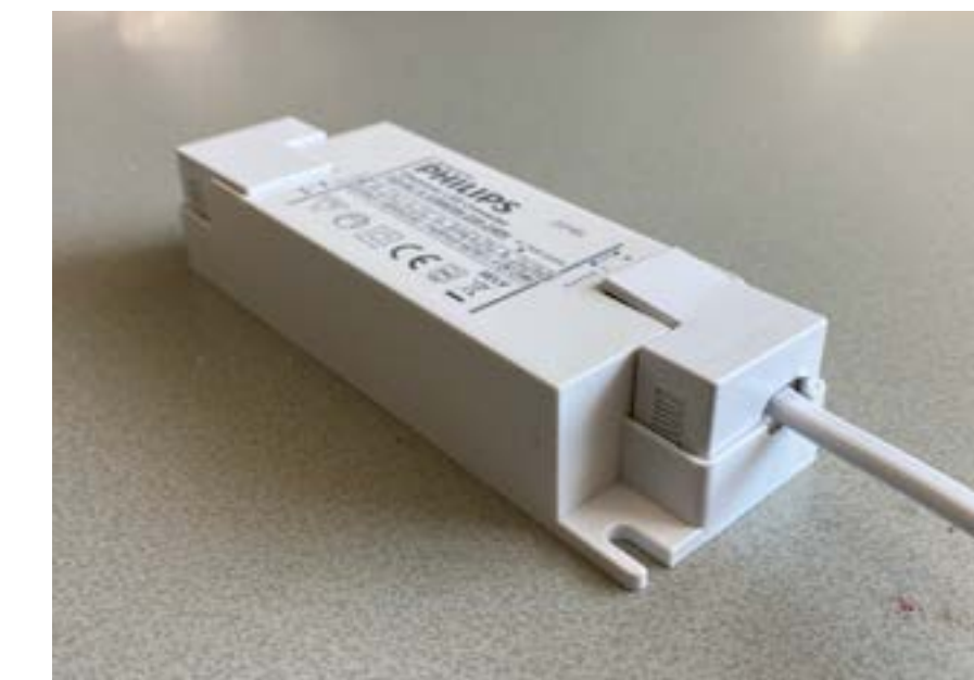
Figure 39. Screwless cable securement in Ledinaire driver.
