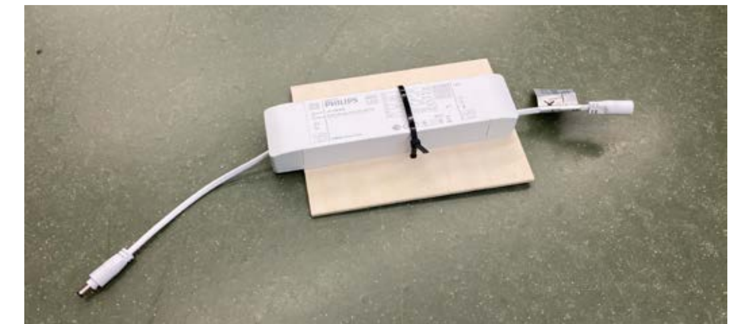
Figure 74. Prototyping the driver to backplate securement by means of a tie wrap.
