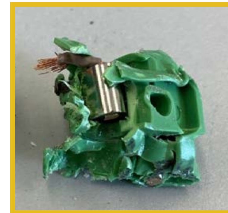
Figure 42. Metal components still stuck in connector plastic in CoreLine.
