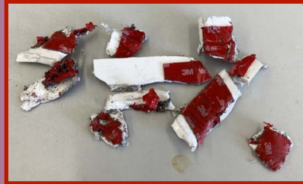
Figure 73. Mixed fragments of PC and rubber sticker.
