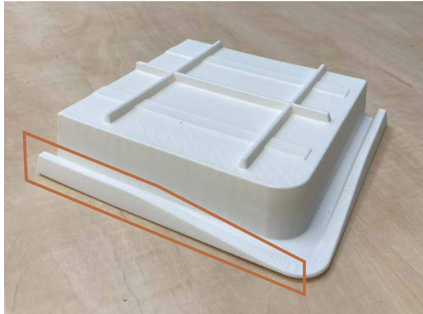
Figure 103. Mold of the corner of the backplate with a very gradual transition from the outer edge and the base of the mold (outlined in brown).
