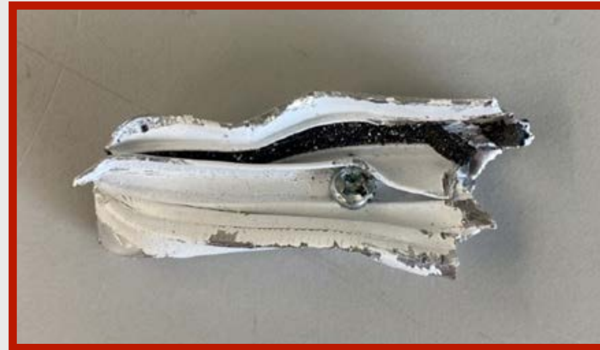
Figure 28. Steel screw that was not liberated from the aluminum frame during shredding of the CoreLine.
