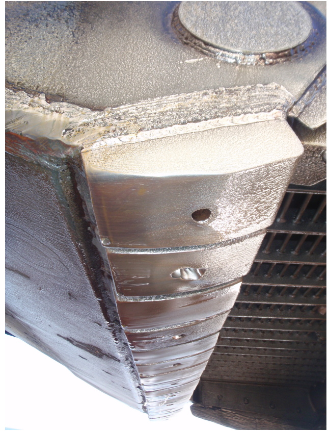
Figure 5.4: The heel jet blocks of a Wild Dragon draghead
