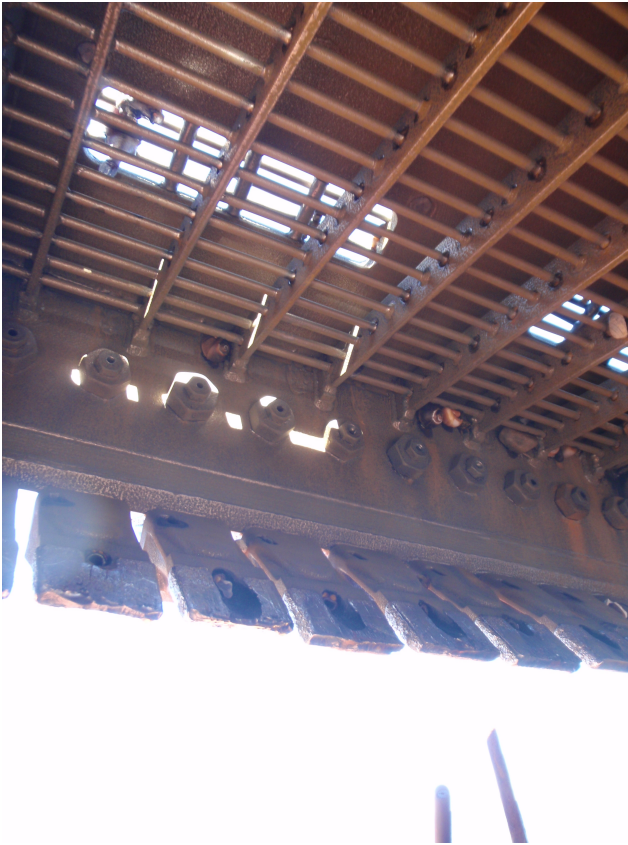
Figure 5.3: The inside of a visor equipped with MEC screening. Behind the MEC screening a water port is visible. Furthermore the visor jets and tooth jets are clearly visible
