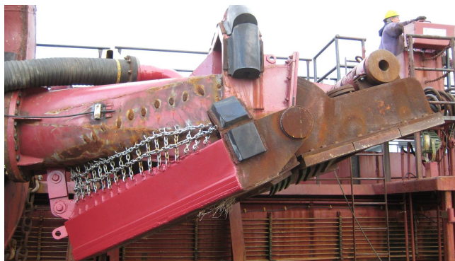
Figure H.1: A turtle exclusion device (bright red) mounted on a draghead
