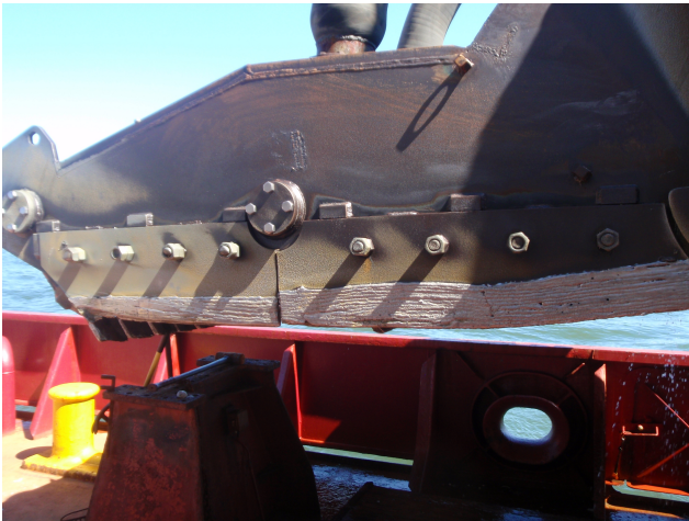
Figure 5.1: A side view of a real Wild Dragon extended visor
