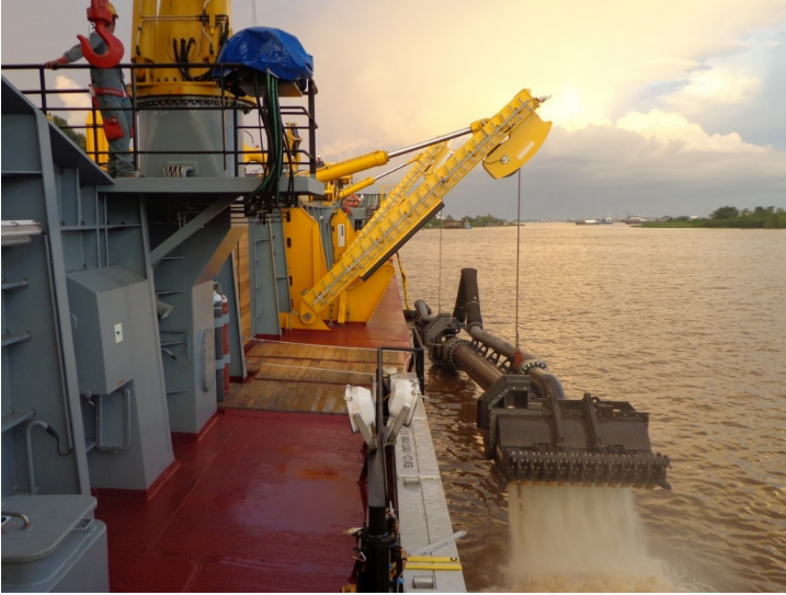
Figure 2.3: Davits supporting the drag arm (Original from: products.damen.com )
