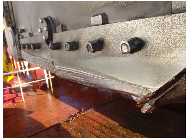
Figure 5.2: The side plates of a draghead with wear due to sand clearly visible
