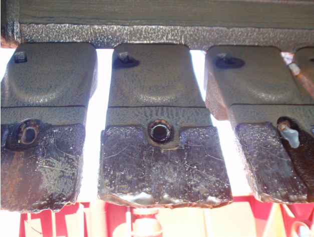
Figure 3.9: Tooth jet nozzles in the teeth of a Wild Dragon draghead
