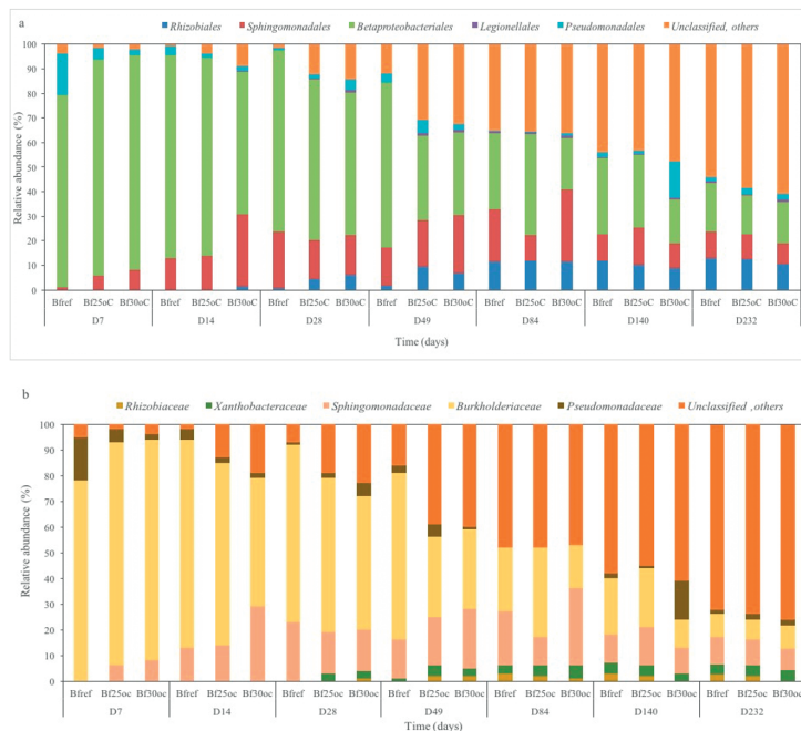
Figure 3.5: Microbiome of biofilms shown as relative abundances (%) of core microbial groups, at both Order (a) and Family (b) level of taxonomic classification, from three sampling locations, developed within pilot distribution systems ( Bf_{ref} = biofilm from reference system, Bf_{25\text{ }^{\circ}\text{C}} = biofilm formed after cold recovery ( T_{max} = 25\text{ }^{\circ}\text{C} ), Bf_{30\text{ }^{\circ}\text{C}} = biofilm formed after cold recovery ( T_{max} = 30\text{ }^{\circ}\text{C} )).
