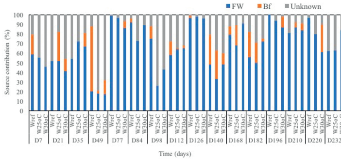
Figure 3.8: The results of source tracker method, showing percent contributions of microbial communities from different sources (feed water =FW, biofilm from relevant pilot DS=Bf, Unkown sources) into sinks ( W_{ref} = water from reference system, W_{25^{\circ}C} = water after cold recovery ( T_{max} = 25^{\circ}C ), W_{30^{\circ}C} = water after cold recovery ( T_{max} = 30^{\circ}C )) on each water sampling day.
