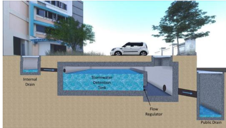
Figure 20 An example of the on-site storm water detention tank [18]
