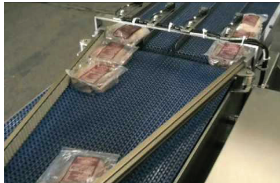
Figure 34 - Multilane singulator unscrambler ; packages enter on multiple conveyor lanes and are redirected to one lane by controlling the entering conveyors in sequence (waldropproducts, 2009).
