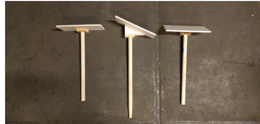
Figure 44 - Wooden prototype pushers to validate the feasibility of the concept; straight, yawed, pitched.
