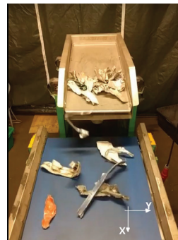
Figure 38 - Still of the video footage used for analysis; Scrap falls off the vibrating feeder onto the conveyor belt which moves in the positive x-direction.
