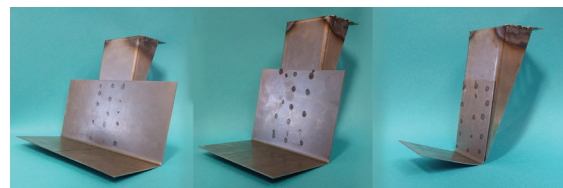
Figure 82 - Three different Gripper prototypes with three different widths. Left: Gripper with a width of 250 [mm]. Middle: Gripper width: 160 [mm]. Right: Gripper width: 80 [mm].
