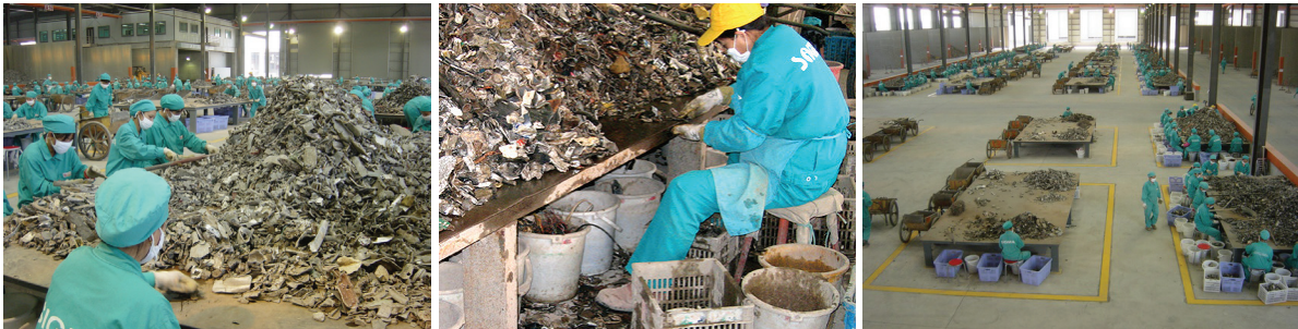
Figure 18 - Handsorting of aluminium scrap. Chinese workers are sorting aluminium scrap by hand. In large factory halls they are sorting 0.5 tonne per person per day. (Courtesy: Minter, 2011b; Bloomberg, 2009)
