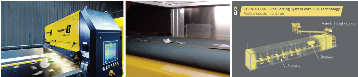
Figure 20 - Steinert aluminium sorting system using LIBS. Steinert sorts small aluminium fractions using laser-induced breakdown spectroscopy for classification. The aluminium pieces are shot off the belt using air pulses (Courtesy: Baum Publications, 2019; Recycling Today, 2016; Steinert global, 2018).
