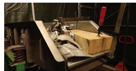
Figure 39 - Using a wooden block to narrow the output of the vibrating feeder, in order to singulate pieces. Result: Pieces got stuck in the feeder.
