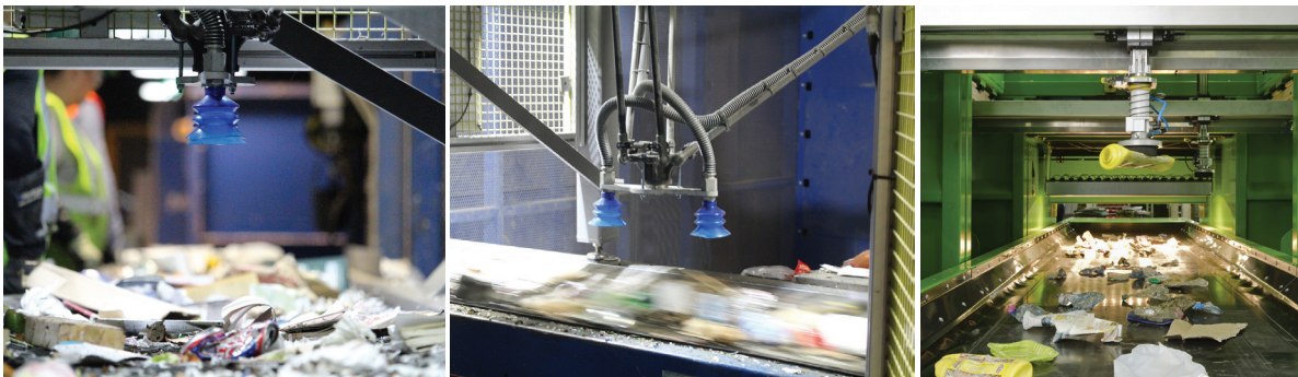
Figure 21 - Vacuum grippers sorting light fractions of plastic and drinking cartons (Courtesy: AMP Robotics, 2018; Bollegraaf Recycling Machinery BV, n.d.)
