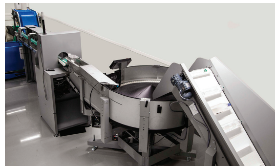
Figure 31 - Unscrambler; water bottles are transported into the machine in batches and exit in a line one at the time (Tomra, 2017).
