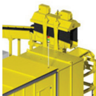
Figure 37 - Singulator for sorting aluminium scrap by Steinert. Scrap comes in from the left and is fed in a vibrating feeder (black), falls into a perpendicular vibrating feeder. (Steinert global, 2019)
