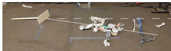
Figure 47 - Result of yawed pusher; pieces are approximately 15 degrees off center when pushed with a pusher under an angle of 30 degrees.
