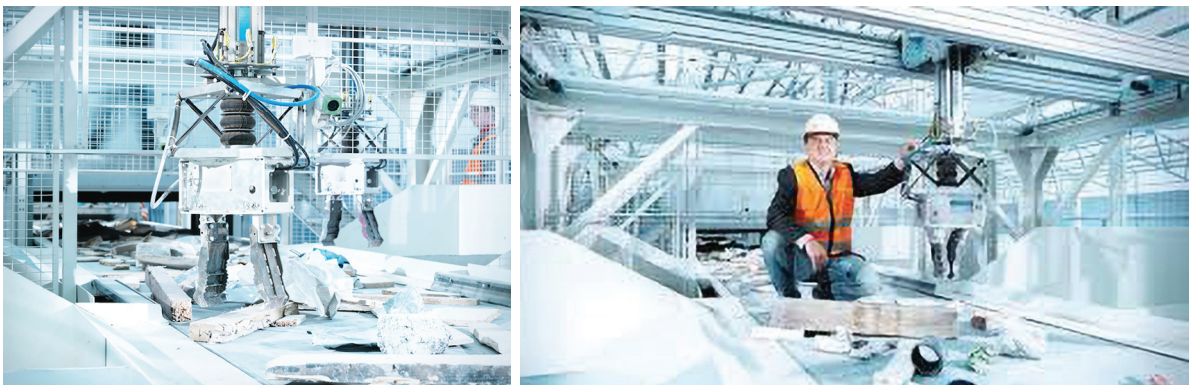
Figure 19 - ZenRobotics sorting system for sorting different construction waste with a robotic system. The system can sort up to 8 ton/hour. (Courtesy: ZenRobotics, 2018b)
