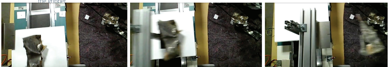
Figure 94 - A piece of scrap is pushed of the white cart and moves perpendicular to the moving direction of the cart.
