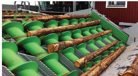
Figure 35 - Screw unscrambler; Trees enter on the right while a screw is rotating. This screw scoops the trees up and transports them one by one upwards (Hein, 2015).
