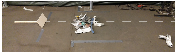
Figure 48 - Result of pitched pusher; pieces are on line with the center of the pusher.
