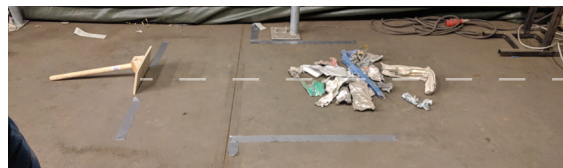
Figure 46 - Result of pitched pusher; pieces are on line with the center of the pusher.
