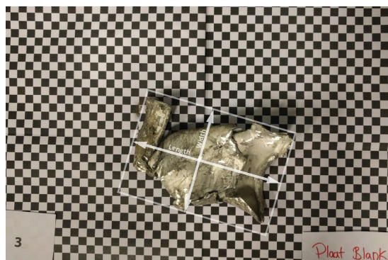
Figure 14 - Sample placed on a blocked background for dimension reference; a box is drawn around the piece of scrap to determine the length and width.
