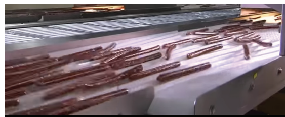
Figure 33 - Vibrating ZigZag; sausages enter on the left and by vibrating a sharkteeth-like surface, the sausage align (ABB Robotics, 2010).
