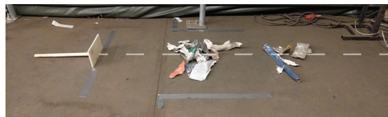
Figure 45 - Result of straight pusher; pieces being pushed forward and aligned around the center of the pusher.
