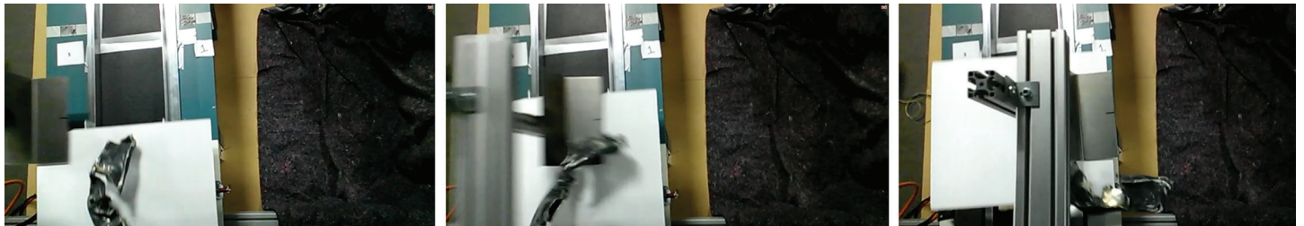
Figure 93 - Testing the sliding cart propelled by a remote car. (1) The piece is moved forward (upwards in the figure), (2) the Gripper moves sideways but moves too early, (3) the piece is moved sideways but not enough and will be moving back onto the gripper
