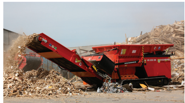
Figure 9 - Hammel; the shredding machine Reukema uses to shred the aluminium into smaller pieces. (Courtesy: https://www.hammel.de/index.php/en/unternehmen-en/uber-hammel-en )
