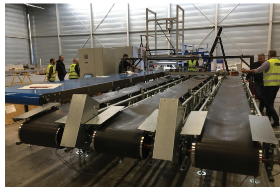
Figure 78 - Testing setup built at ARCO solutions for Reukema. One large conveyor belt (blue) transports scrap. The material is pushed off the belt to a perpendicular belt, from which it is pushed on one of the trog conveyor belts.
