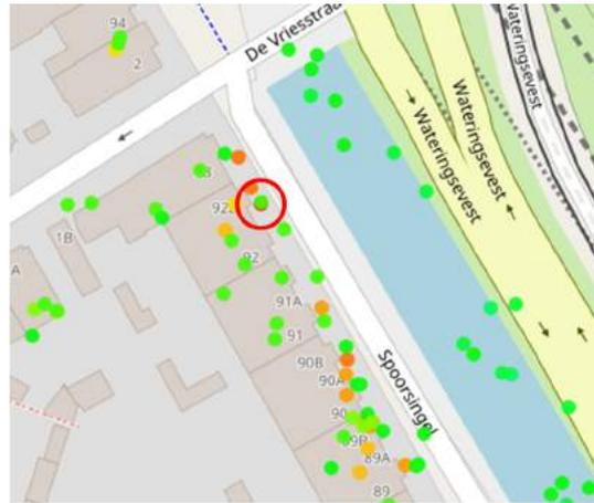
Figure 6.9: InSAR data points in the northern part of the project area of the descending track of both the 2 year and 9 year dataset. A data point is indicated in both datasets which has almost exactly the same position.
