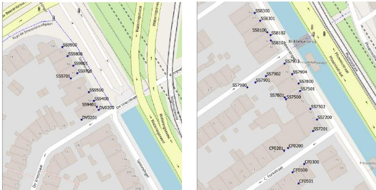
Figure 6.2: Positions of the levelling benchmarks
