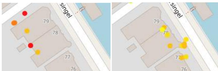
Figure 6.12: InSAR points on buildings Spoor singel 78 and 79 of the ascending (left) and descending (right) track
