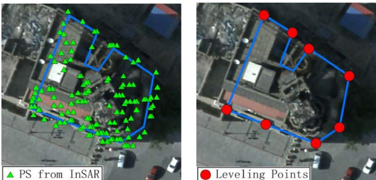
Figure 4.9: Location of PS (left) and location of levelling points (right) on the Bohai Building
