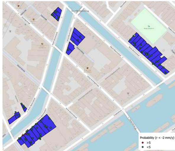
Figure 5.19: Probability of a deformation rate of more than  $-2$  mm/y based on the calculated  $\sigma_r$  of each InSAR point for InSAR data between January 2013 and December 2016
