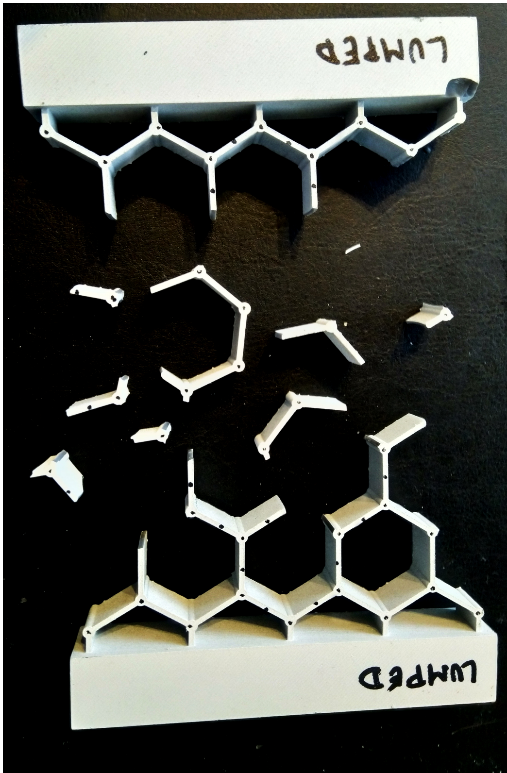
Fig. 9.10 Photograph of the lumped-node honeycomb post-experiment fragments
