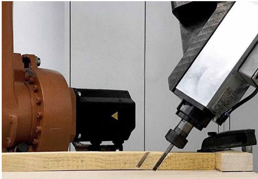
FIG. 5.18 Two methods of toolpath generation for material removal: Layer by Layer removal on the top and perimeter removal without crushing the material in the middle and bottom.
