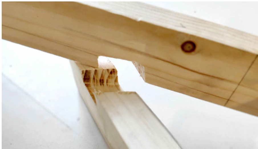
FIG. 5.11 Top: Robotically fabricated prototype of the first two reciprocal cells; Bottom: a reciprocal connection in which the notches are introduced on both members.
