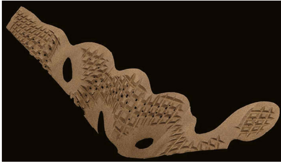
FIG. 4.12 Unrolled patch of cork components, Cork gains intended flexibility and double curved bending.
