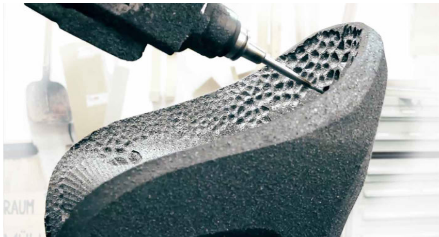
FIG. 4.31 Process of milling the cell in higher resolution perpendicular to the geometry that results in a refined surface quality and increases the friction between two materials.
