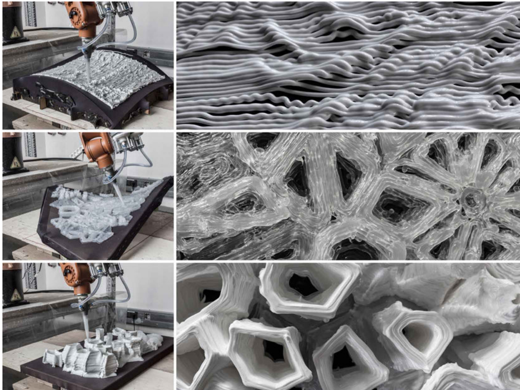
FIG. 4.23 Robotic silicone printing experiments, linear continuous printing (top); cellular printing on a free form fabric (middle); prototype testing height, cantilevering and size ranges (bottom).
