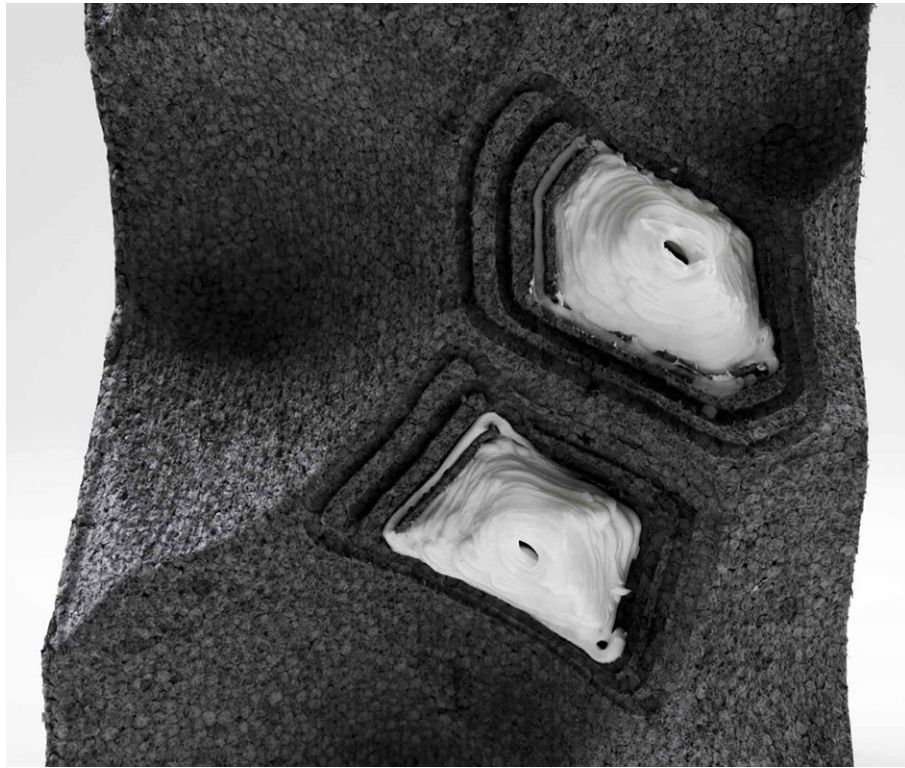
FIG. 4.24 A test sample as a proof of concept prototype integrating subtractive robotic manufacturing applied on EPS and additive deposition of silicone with robotic arm.
