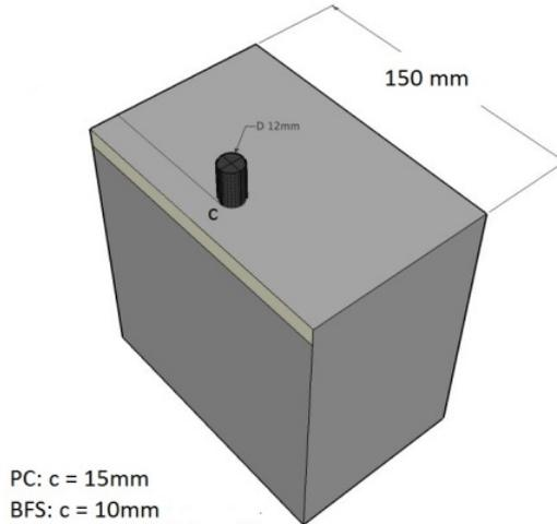
Figure 3. Geometry of reinforced concrete specimens
