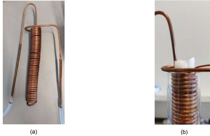
Figure 4.5: (a) Cold finger (b) Rolled plastic foam sheet to prevent vapour losses
