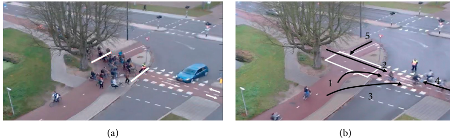
FIGURE 3: Example of the video data (a) with the waiting area defined by the white lines. The black arrows indicate different directions in which additional cyclists can influence the queue discharge process (b).
