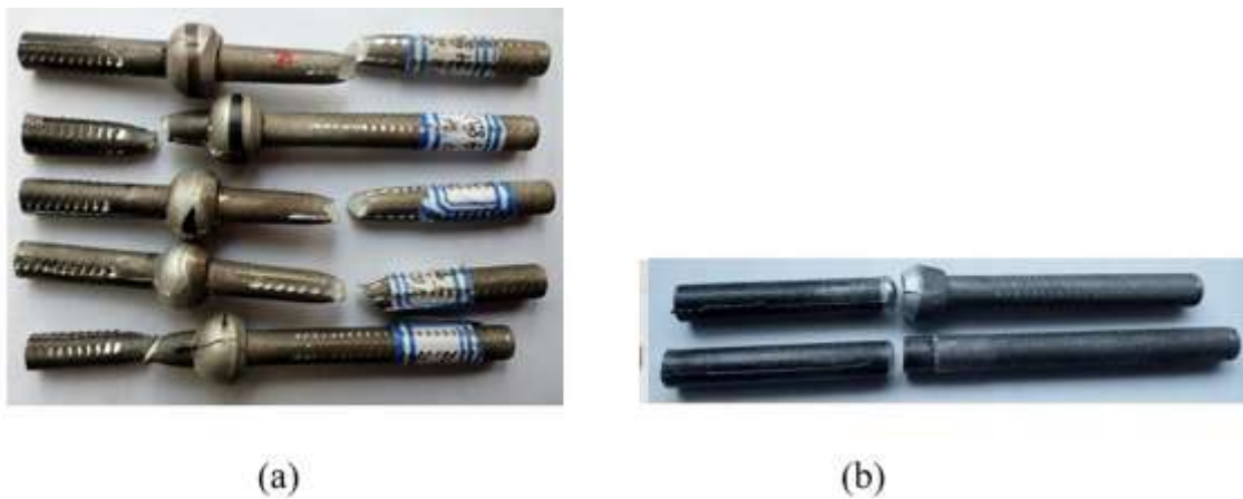
Fig. 2. Barreled samples (a) and deformation and bonding inside the welding chamber at punch displacements of 6 (b), 12 (c), and 24 mm (d) ( v = 0.8 \text{ mm/s} ; T = 440_{\text{C}} ).
