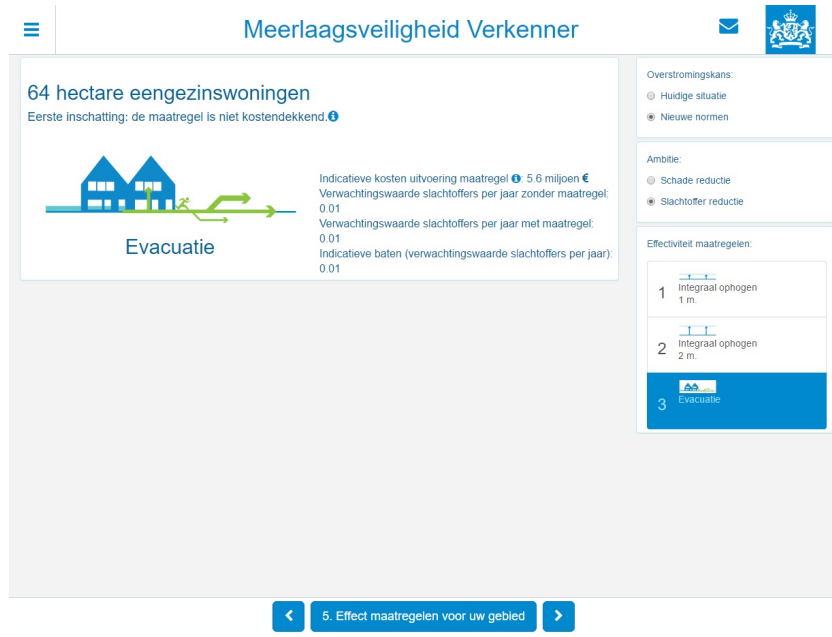
Figure C.36: Results for victim reduction after measures that make evacuation easier, in case that the new norms have been established.
