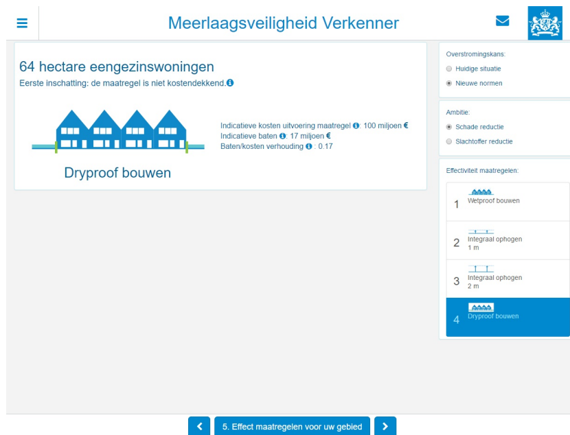
Figure C.33: Results for financial damage reduction after dryproof building measures, in case that the new norms have been established.
