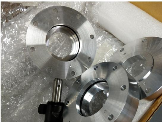
(a) O-ring installed and mounted on optical post
