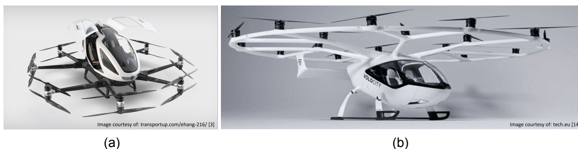
Figure 1.1: A comparison of two UAM designs, the (a) Ehang 216F [4] and the (b) Volocopter VoloCity [5], which have approximately the same cabin but different planform volumes.
