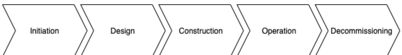
Figure 1.2 Lifecycle of Construction Project
