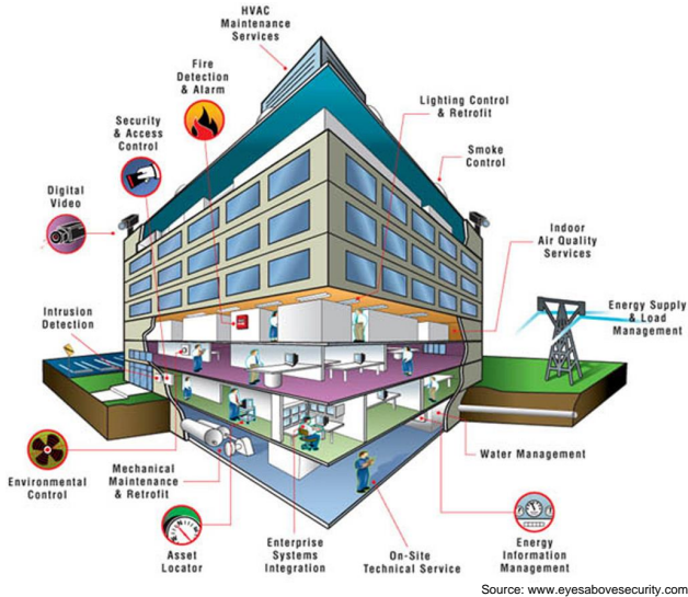
Figure 1.2: Illustration of various wireless sensor nodes in a smart building (courtesy of Eyes Above Security Systems Inc.).
