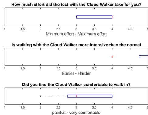
**Figure 4-10:** Results of the evaluation questionnaire. The test was found to take quite some effort. It was definitely more intensive than normal walking. The Cloud Walker felt uncomfortable to walk in.
