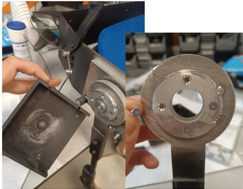
(a) Left hip; Damage in the cap caused by the cable and cable clamps. (b) Left joint; loose screws and smoothed edges caused by cable clamps.
