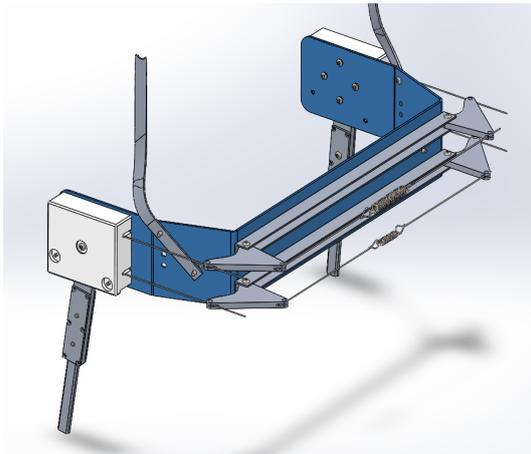
**Figure 2-5:** In blue: Stainless steel hip plate functioning as a base for all other parts.
