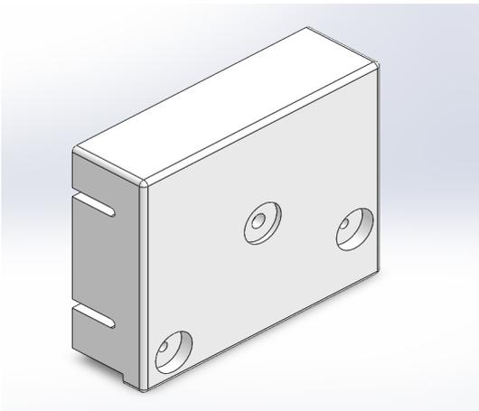
**(b)** latest version of the cap with slots at the side, which still guide the cables, but also makes it easier to assemble and disassemble.
