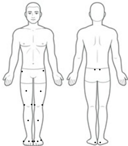
**Figure 3-1:** The black dots are the markers placed over the lower body. The dots on the center front of the upper and lower leg became marker clusters in the actual test.
