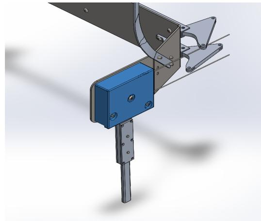
**Figure 2-7:** In blue: PLA printed cap covering the rotating parts of the hip joint.
