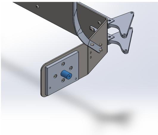
**Figure 2-6:** In blue: The aluminium axis of the hip joint created on the metal lathe.
