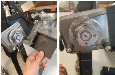
(c) Right hip; Damage in the cap caused by the cable and cable clamps. (d) Right joint; Smoothed edges caused by cable clamps.
