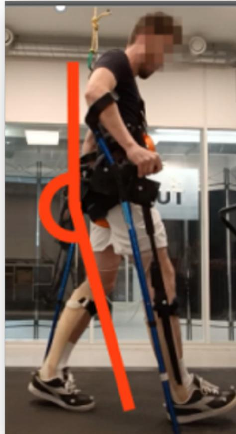
**Figure 2-3:** Flexing the upper body will put tension in the lower spring at the back of the Cloud Walker. The tension will extend the hip of the standing leg, creating a larger step.
