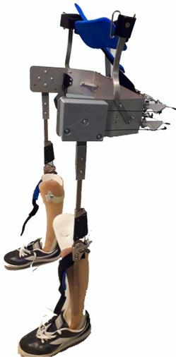
**Figure 2-1:** The complete side view of the final first prototype of the Cloud Walker. The leg parts and waist fixation are from an ARGO. The hip frame is self designed.
