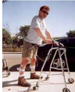
**Figure 4-2:** The electrodes of the Parastep© by Sigmedics are controlled by the controller in the walker
