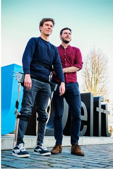
**Figure 1-1:** The Cloud Walker is worn by the participant on the left. For safety reasons, there should always be someone near in case the user is about to fall.
