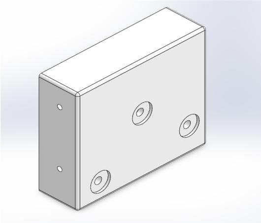
**(a)** first version of the cap with small holes at the side to guide the cables.
