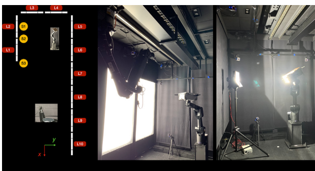
Fig. 4. Visualization of the TRON facility for the generation of the SPEED+ images. Light boxes (L1 - L10) and sunlamp locations (S1 - S3) are noted Park et al. (2021a).
