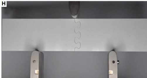
Figure 11 3 three-point bending setup with specimen (14)
