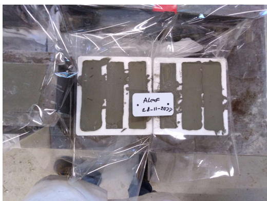
Figure 36 small prisms for compressive and bending resistance tests
