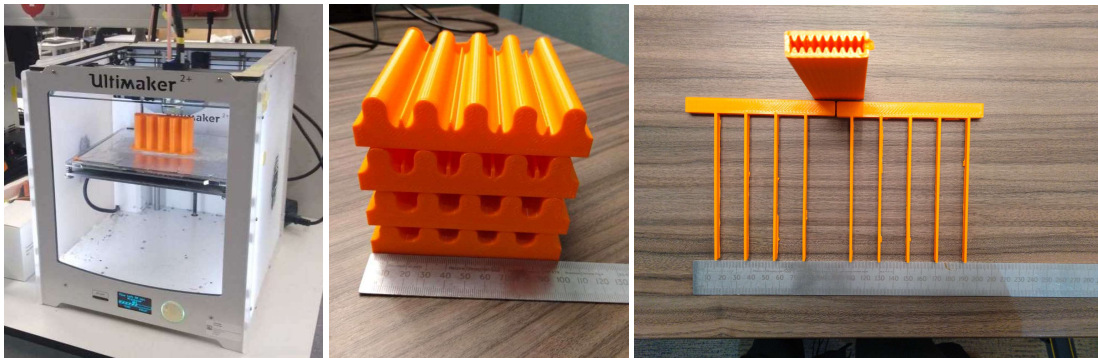
Figure 33 Production and results of the 3D printed mould. Left is the 3D printer, in the middle are the moulds for the tabs and right are the moulds for the gaps.
