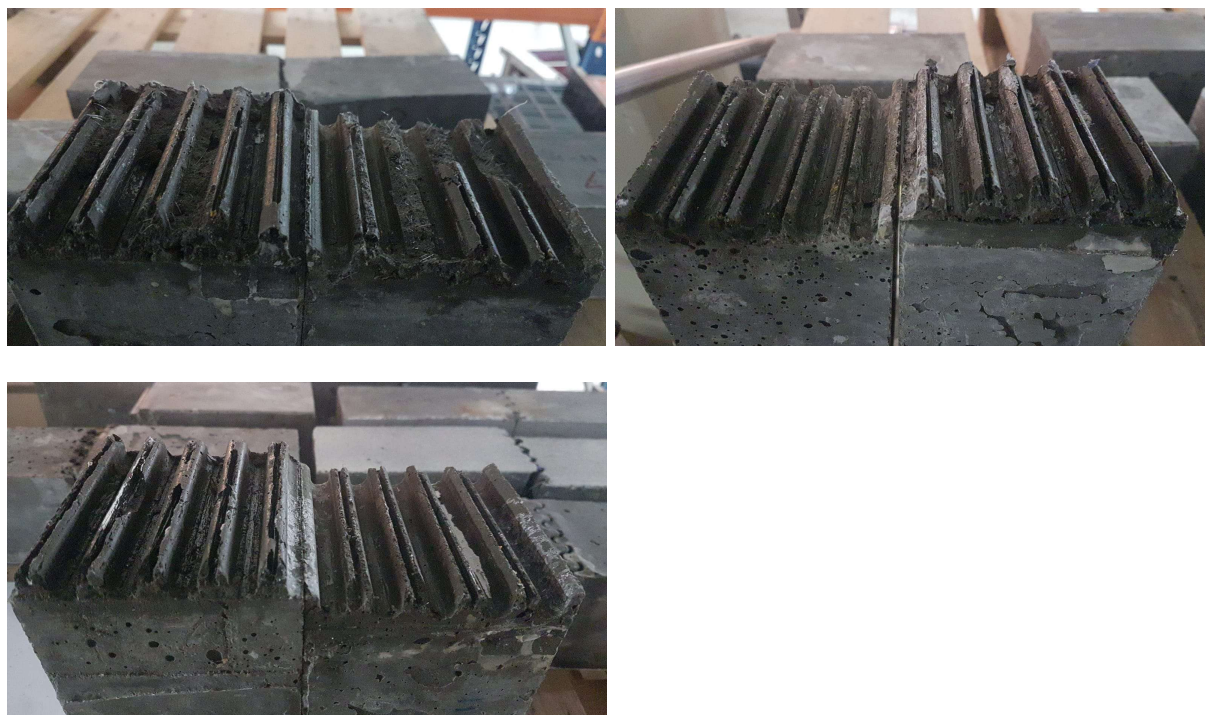
Figure 124 Design 3 taken apart after testing. Where the picture on the top left is sample 5, the picture on the top right is sample 6 and the picture on the bottom left is sample 7.
