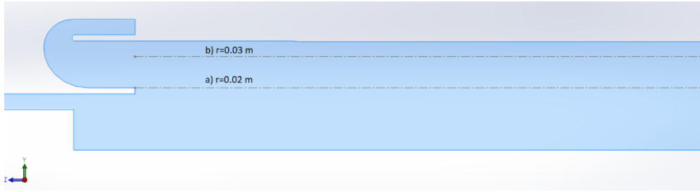
Figure 4.3: Geometry of the TU Delft's FlameSheet™ burner fluid domain used for the CFD simulation. Axial lines at r=0.02 m and r=0.03 m are used for the mesh independence analysis.
