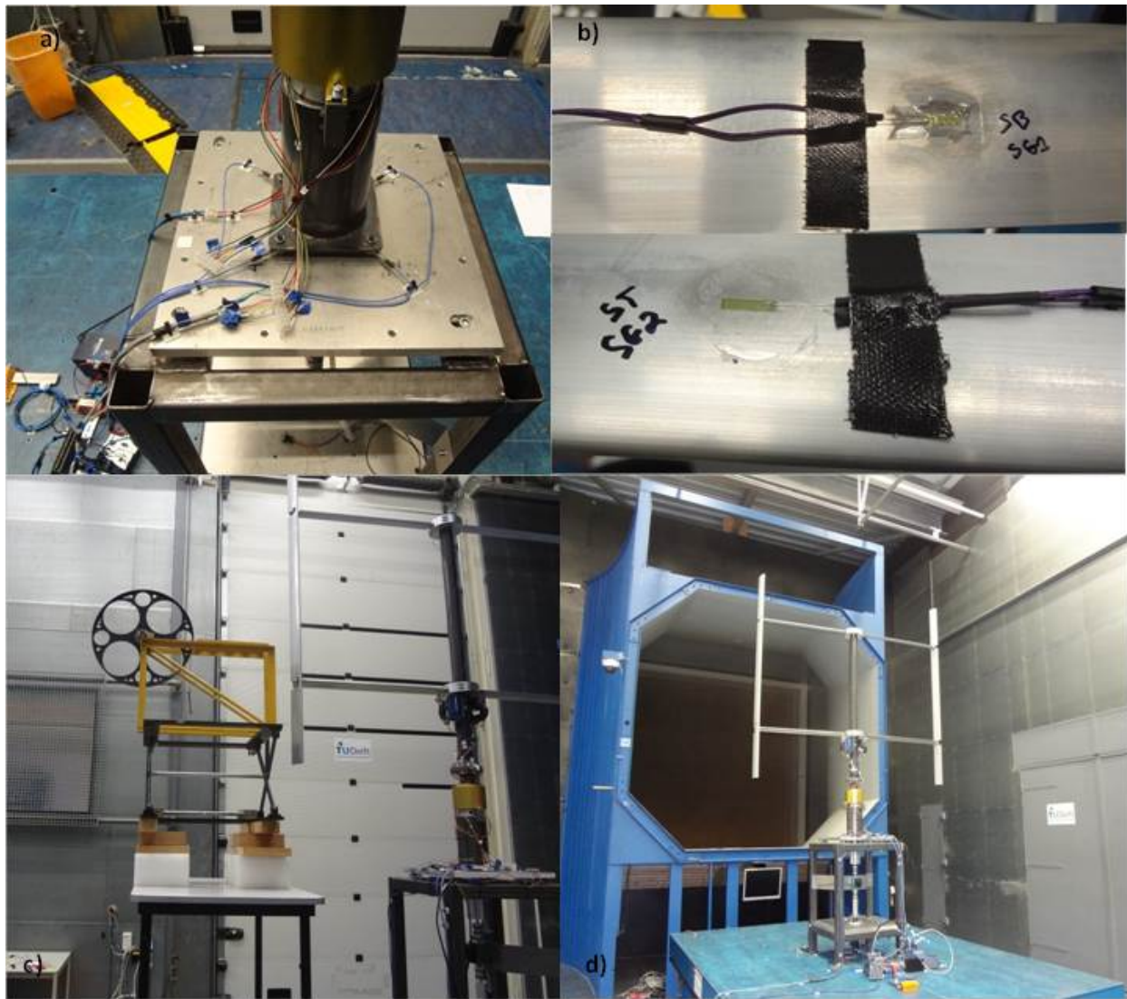
Figure 6: Photos of the installed PitchVAWT Turbine a) Load Cells with wiring b) Installed strut strain gages c) calibration rig for strain gages, d) PitchVAWT in the OJF Facility at TU Delft.
