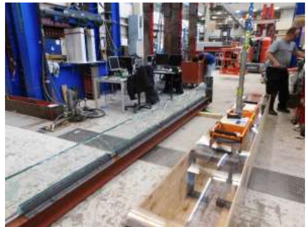
Fig. 6: Damaged specimen siliconed into steel profile which simulates the lateral support of the façade glazing in the real structure
