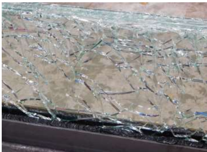
Fig. 13: Part of specimen 2 after having 3 plies damaged. Note the overlapping cracks in successive plies
