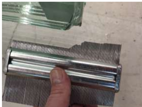
Fig. 5: Measurement of damage using a contour gauge
