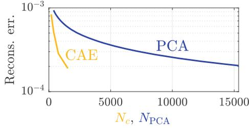
**Fig. 4.** Reconstruction error with a PCA-based method (blue) and the autoencoder (yellow) for different dimensions of the latent space,  $N_c$ , or number of retained PCA components,  $N_{PCA}$ . The reconstruction error is computed as the mean squared error between the reconstructed velocity field and the exact field, averaged over the test set. (Color figure online)
