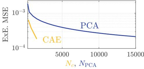
**Fig. 5.** Reconstruction error on the extreme events flow states with PCA-based method (blue) and autoencoder (yellow) for different dimensions of the latent space,  $N_c$ , or number of retained PCA components,  $N_{PCA}$ . The reconstruction error is computed as in Fig. 4 but only on the flow state corresponding to extreme events. (Color figure online)
