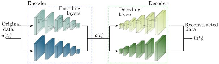
**Fig. 2.** Schematic of the 3D multiscale convolutional autoencoder.
