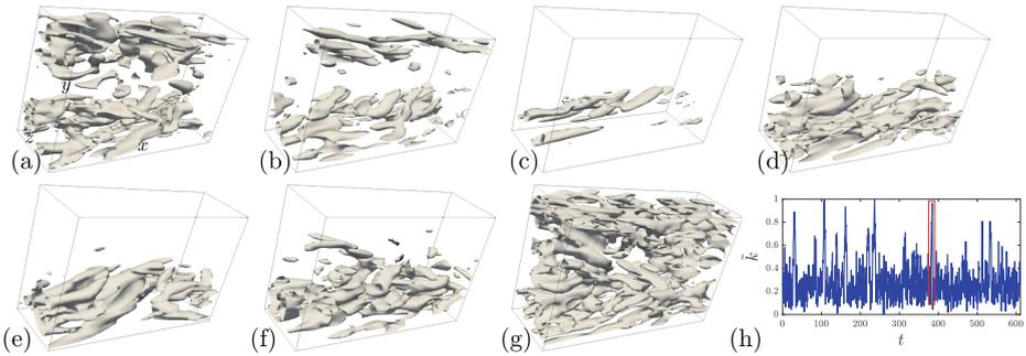
**Fig. 1.** (a–g) Snapshots of the  $Q$ -criterion isosurface (with value  $Q = 0.1$ ) during an extreme event, where  $Q = 0.5(\|\boldsymbol{\omega}\|^2 - \|\mathbf{S}\|^2)$ ,  $\boldsymbol{\omega}$  is the vorticity vector, and  $\mathbf{S}$  is the strain-rate tensor. (h) Evolution of kinetic energy,  $k$ , of the MFU. The red box indicates the event whose evolution is shown in (a–g). (Color figure online)
