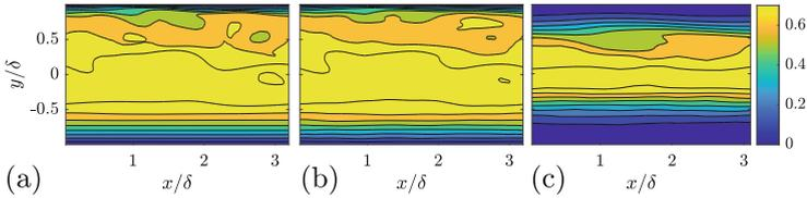
**Fig. 6.** Comparison of (a) the velocity magnitude (ground truth), (b) the CAE-reconstructed velocity magnitude, (c) the PCA-reconstructed velocity magnitude in the mid- $z$  plane for a typical extreme event snapshot in the test set.
