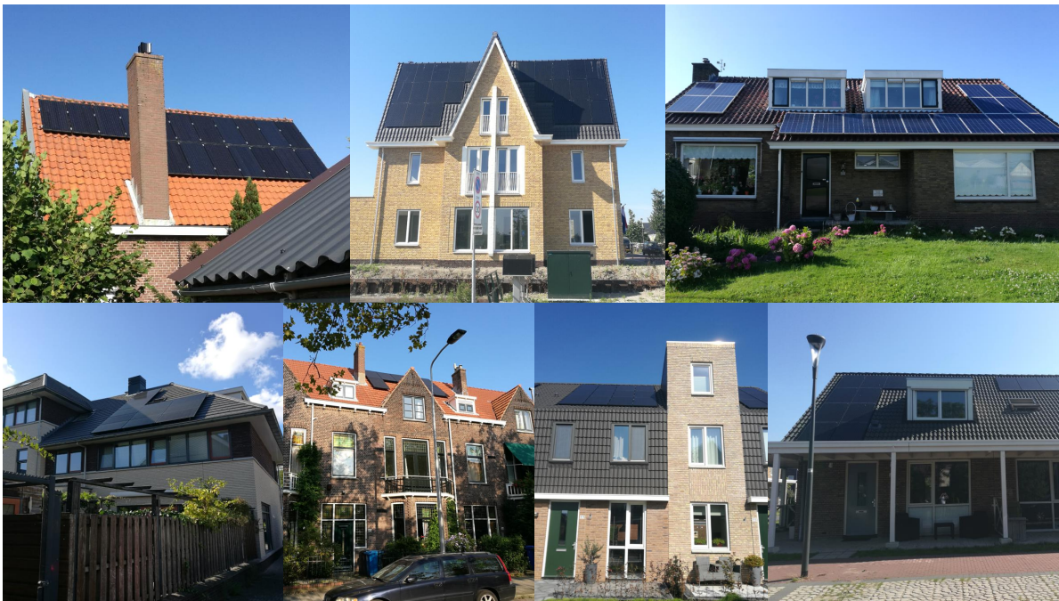
Figure 1.3: Partial shading caused by chimneys, dormers, trees, the shape of the building itself, etc. [5]
