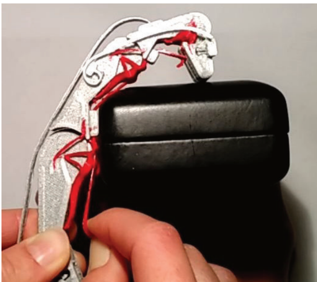
Figure 20: The prototype performing an adaptive grip.
