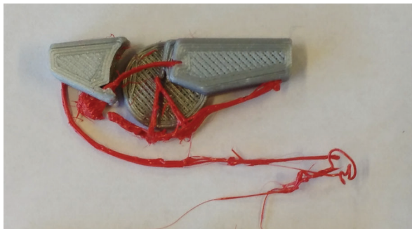
Figure 30: A sample that shows a thin configuration printed with MPflex45 resulting in a failed print. Red is MPflex, grey is PLA.
