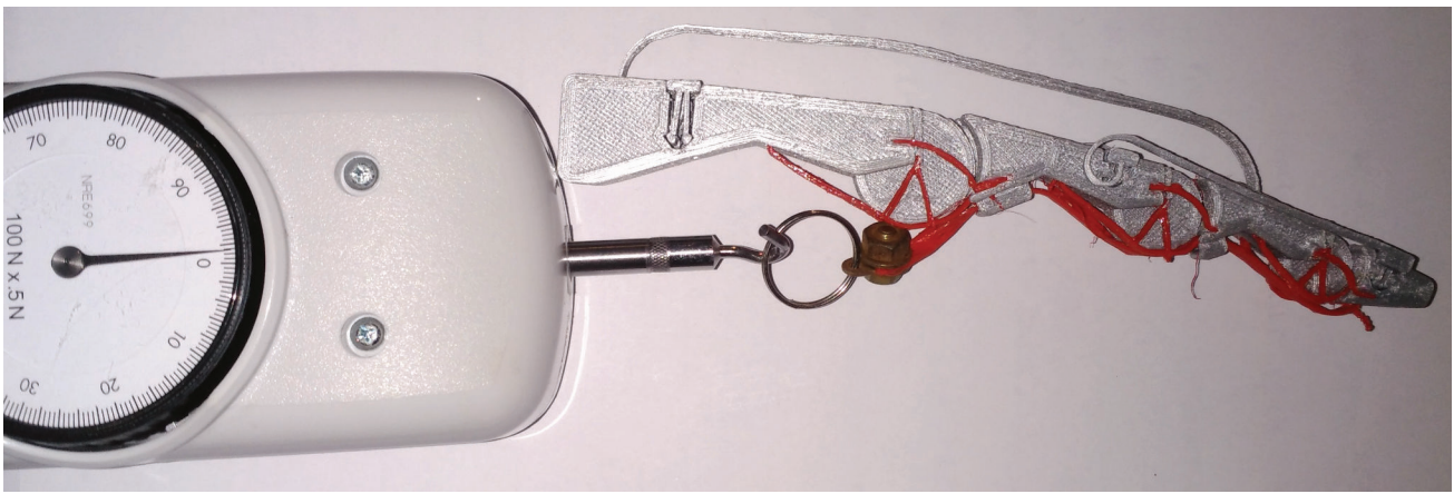
Figure 19: The test set-up to measure the actuation force to bend the finger.
