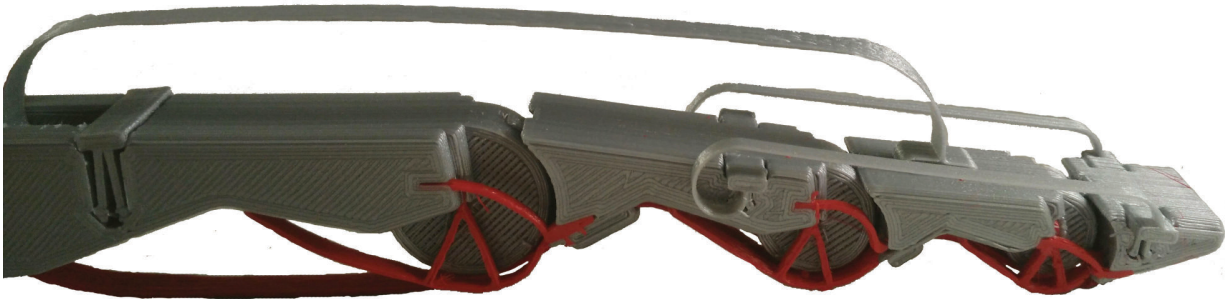
(a) The prototype with the support material before assembly.
