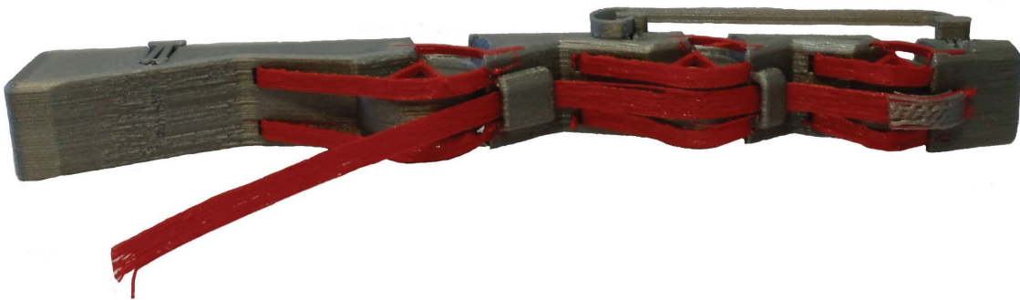
(c) Picture of the prototype showing the pulling cable and the pulleys.
