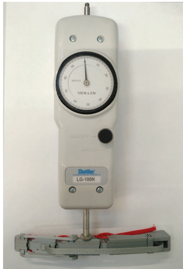
Figure 18: The test set-up to measure the forces exerted at the phalanges when translation in the x-direction occurs.
