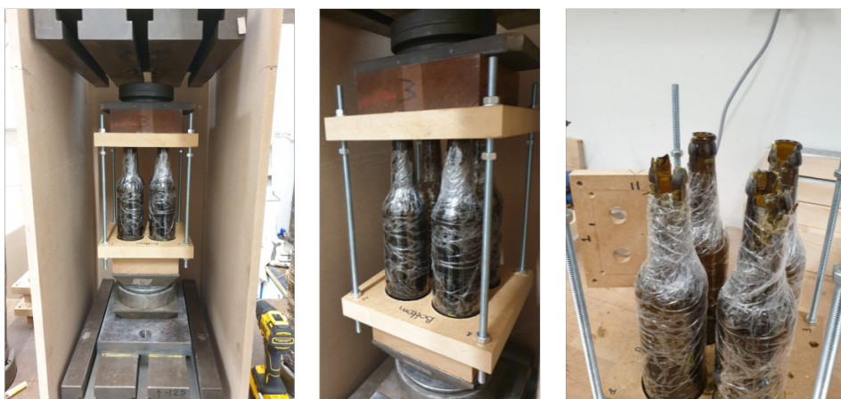
Figure 3 – 'Test 1' configuration set-up before (left and middle) and after testing (right).
