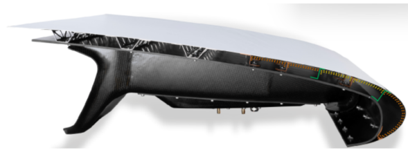
Fig. 6 HLFC suction segment prototype developed in the project HLFCWin [31]
