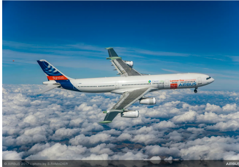
Figure 2.8: Airbus A340 Flight Lab with laminar wing sections during a flight test as part of the BLADE program [34]
