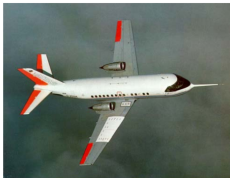
Figure 2.4: DLR VFW614 ATTAS Aircraft in flight test with NLF glove [18]
