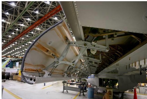
Figure 2.24: Krueger flap on Boeing 747-8 [50]
