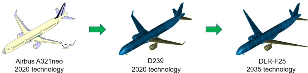
Fig. 4 Aircraft design process from the A321neo reference aircraft to the D239 and the DLR-F25 configurations [33]
