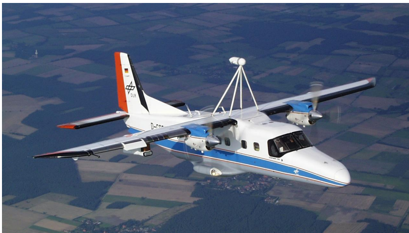
Figure 2.16: DLR Dornier 228 equipped with an HLFC glove and an infrared camera used for transition detection [41]
