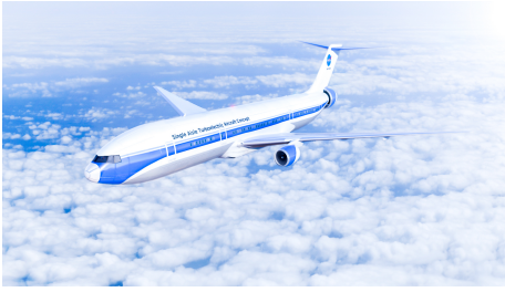
Figure 6.2: Rendering of the NASA STARC-ABL concept [1].
