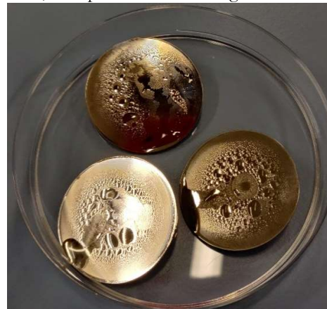
Fig.6-3. Collector plates after \mu -VCM test corresponding to the material of the OF connector protectors.
