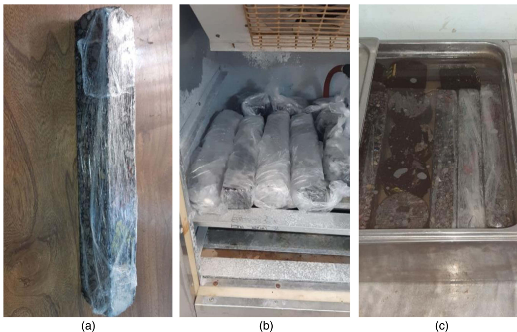
Fig. 5. The F–T cycle process: (a) covering the beam samples after saturating by vacuum; (b) putting in a chamber with 18°C temperature; and (c) putting in a hot water bath with 60°C temperature.
