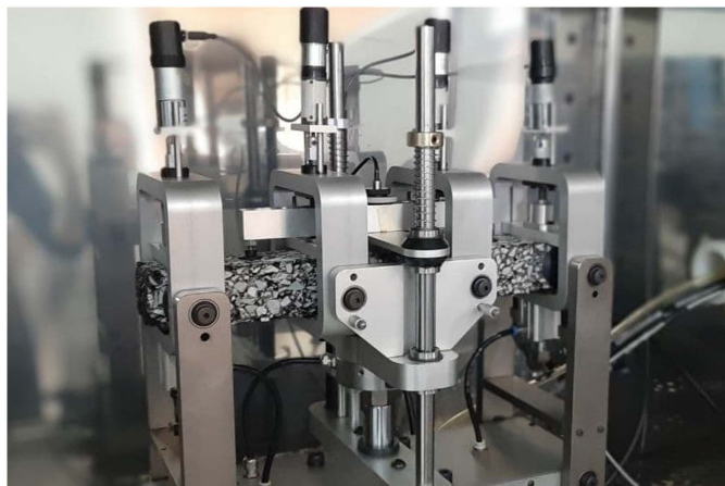
Fig. 7. The beam fatigue test setup.
