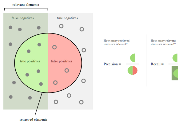
Figure 2.2: Precision and Recall (Edited, https://upload.wikimedia.org/wikipedia/commons/2/26/Precisionrecall.svg by Walber, CC BY-SA 4.0 < https://creativecommons.org/licenses/by-sa/4.0/ >, via Wikimedia Commons)
