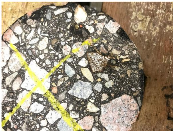
Figure 7 – A piece of metal was found in the specimen during polishing
