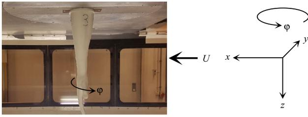
**Fig. 2** A hand model in the wind tunnel test section and the used coordinate system. The yaw angle  $\varphi$  is positive for the thumb leading into the main flow direction, while  $\varphi = 0$  for the hand palm perpendicular to the main flow direction. The model is mounted flush with the force sensor plate, which itself is flush with the upper wall of the test section
