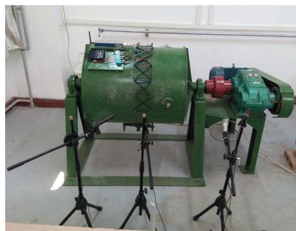
Fig. 5. Ball mill equipment used in the experiments.
