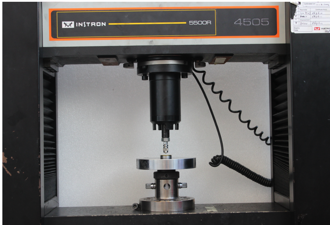
Figure 3.7: Experimental setup for Ball-on-the-Ring
