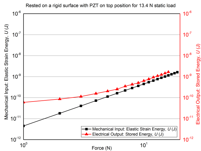
Figure 4.23: Comparison between the mechanical input and electrical output for the boundary condition-1 with the static load of 13.4 N
