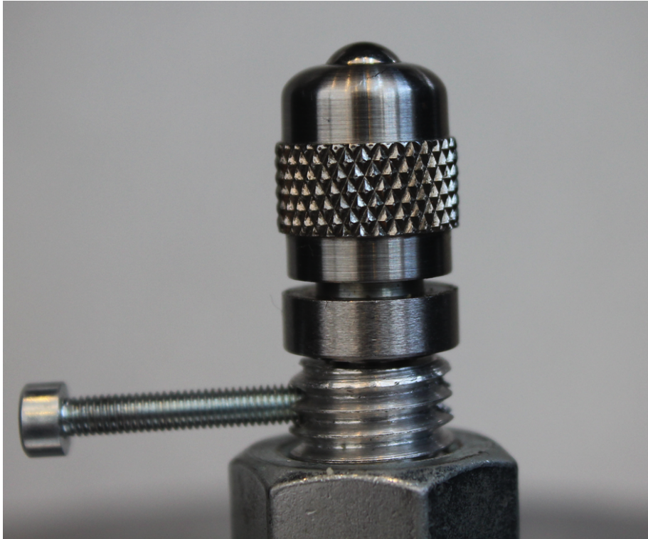
Figure 3.8: The Ball of radius 0.004m used for transferring the load from load cell to piezoelectric buzzer
