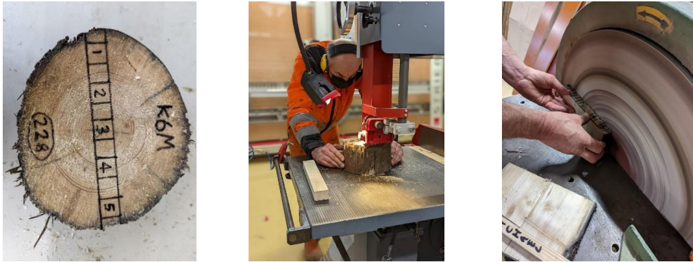
Figure 32 Sample location established, initial cut and sanding.
