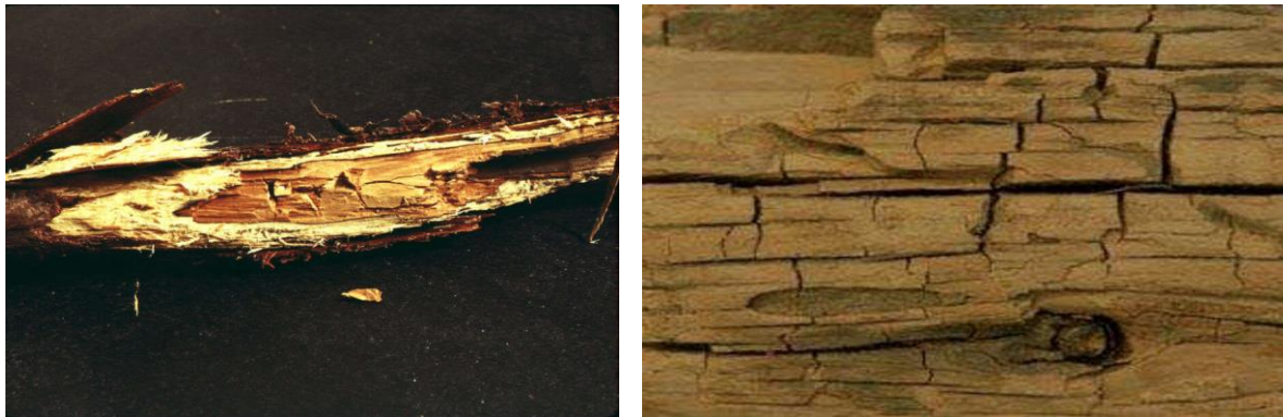
Figure 7 Left - Example of internal brown rot and external white rot. Right – Example of soft rot [18]
