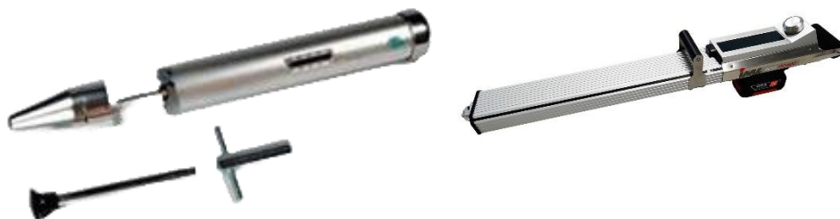
Figure 21 Left - Impact hammers – Pilodyn. Right- IML-RESI PowerDrill [35]
