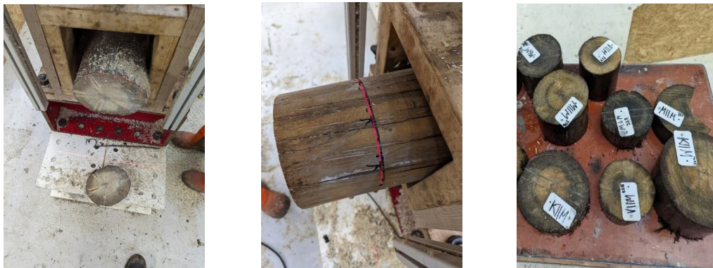
Figure 31 Procedure involving the cutting, preparation, and labelling of cross-sections.
