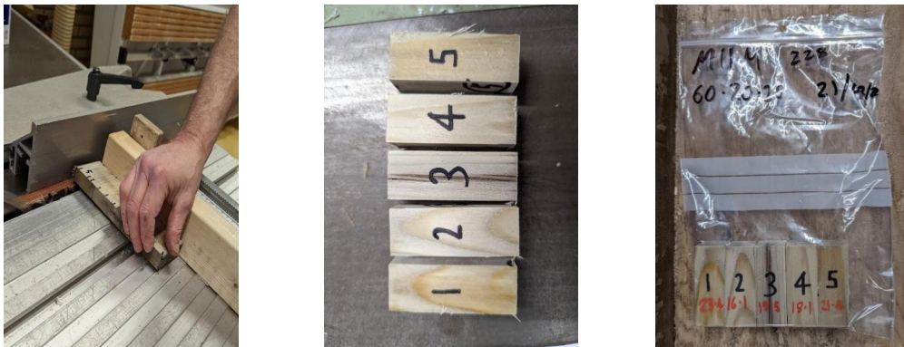
Figure 33 Samples being levelled, final product & plastic wrap to keep moisture content.
