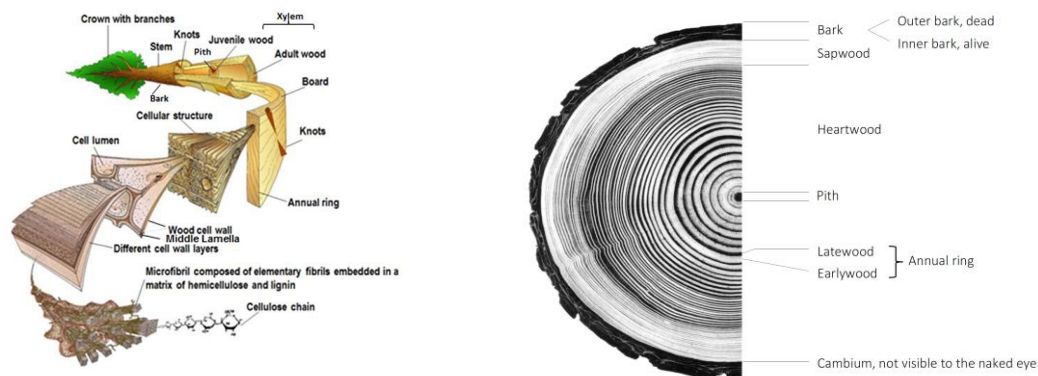
Figure 4 Left - Scheme of the hierarchical structure of coniferous wood (softwood). [9] Cross-section through a coniferous stem, Douglas fir. [10]
