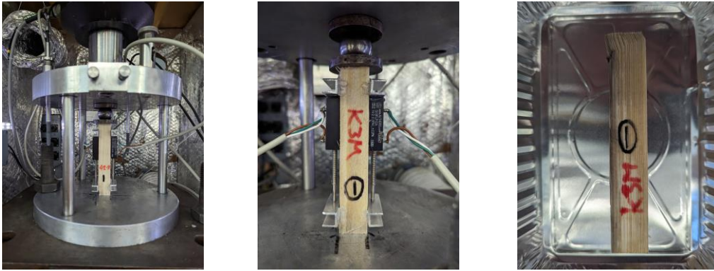
Figure 35 Compression test set-up; Left- compression machine with sample. Middle- K3M with attached LVDTs. Right- Sample after shear failure.
