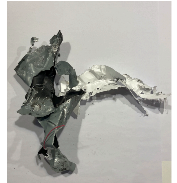
FIGURE 33 Steel folding in reflector sheet
