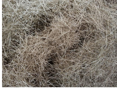
Figure 3.1 Steel fibers in UHPFRC mix [29]
