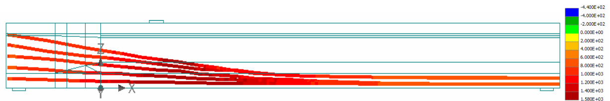
Figure 5.67 Normal stresses \sigma_{xx} in prestressing tendons at failure in T-U0 (MPa).
